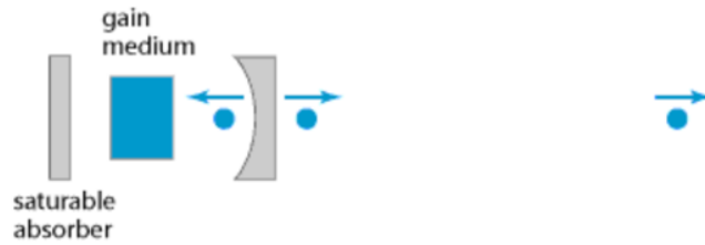
Figure 2.7 Schematic setup of a passively mode-locked laser reprinted from [103].
