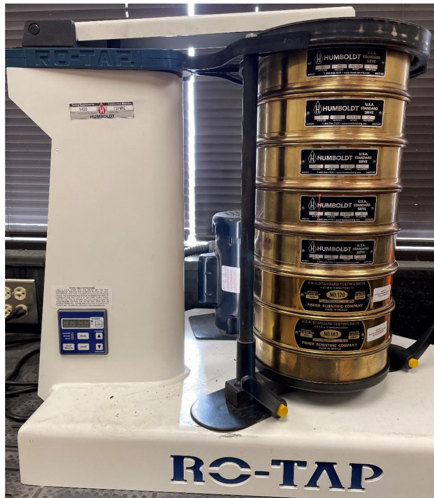
Figure 50. Ro-Tap machine used for proppant sieve analysis.
