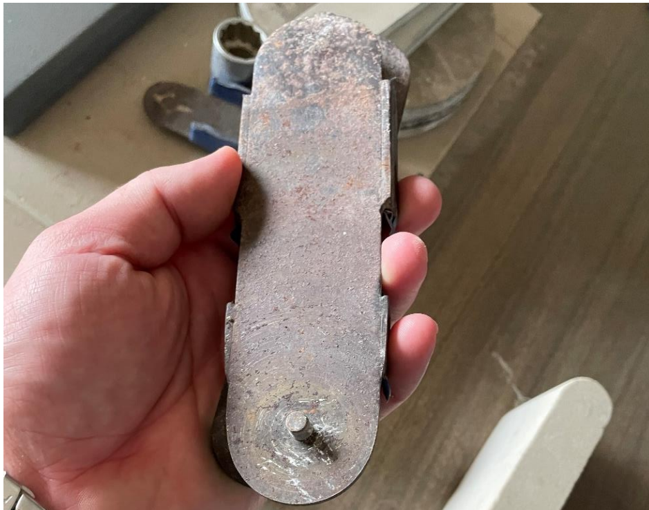
Figure 27. A jig used to create the end radii of the samples.
