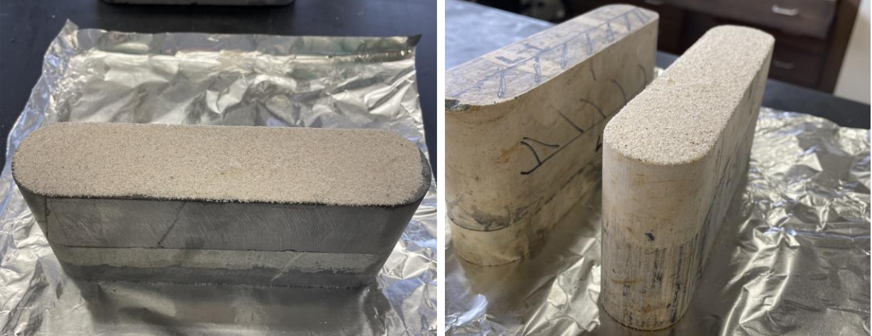
Figure 34. Sample with proppant applied, left - downhole core, right - outcrop.
