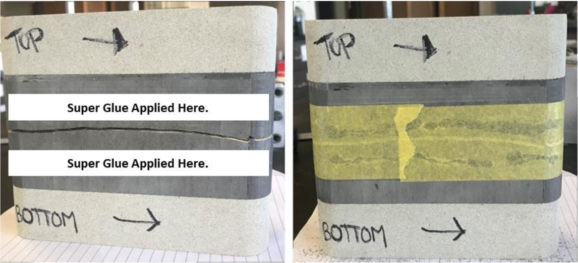
Figure 35. Application of super glue and painter's tape (Modified from Copeland, 2020).
