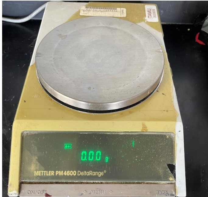
Figure 52. Scale tared to zero, used to weigh proppant for sample preparation and sieve analysis.
