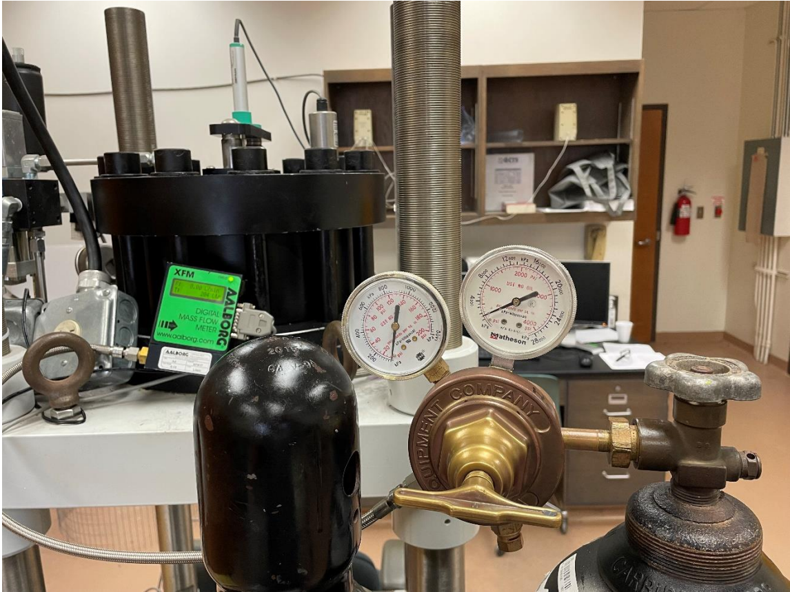
Figure 20. Backside of the experimental apparatus displaying the volumetric flowmeter and spring valve.
