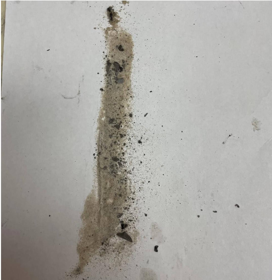
Figure 47. Crushed proppant collection after a fracture conductivity experiment with crushed sample contamination (the dark pieces are crushed pieces of the downhole core sample).
