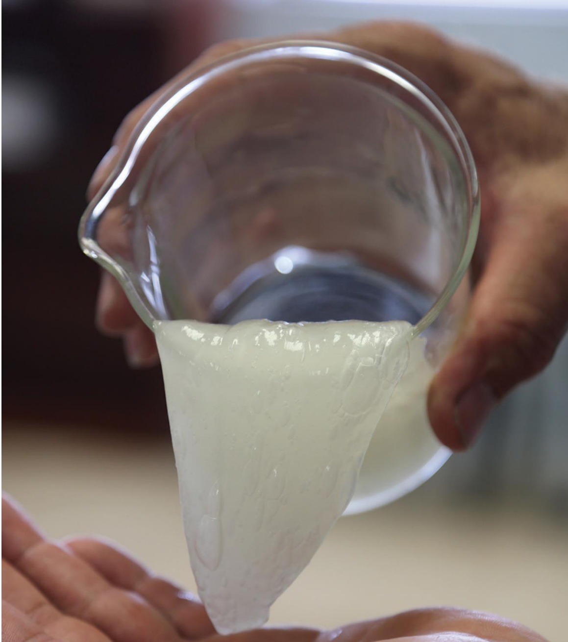
Figure 5. Borate crosslinked gel (Reprinted from Beckwith, 2012).
