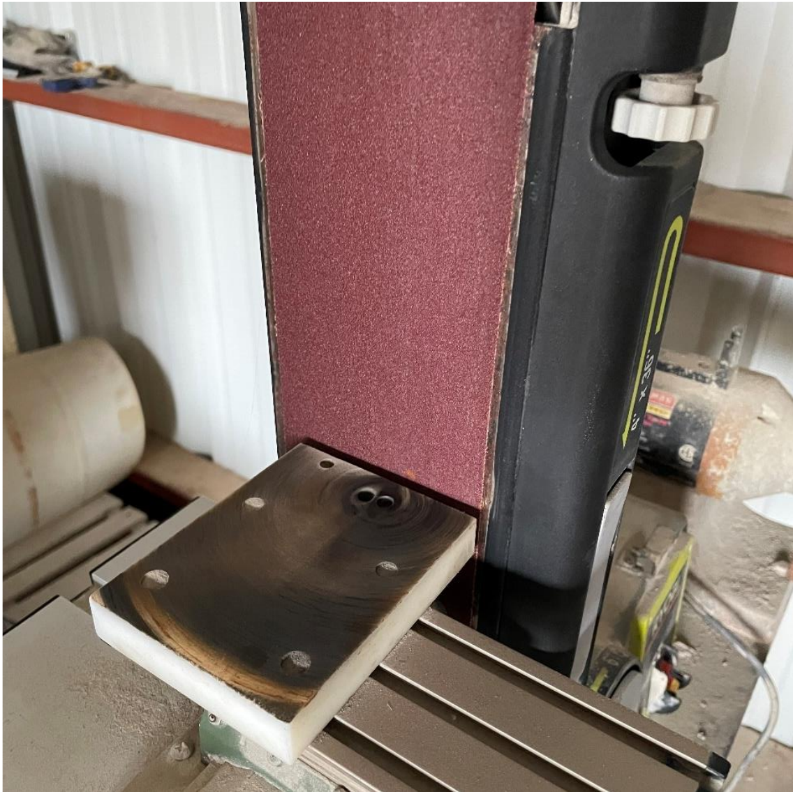
Figure 28. The jig post is inserted into the post hole and a belt sander is used to finish the end radii of the samples.
