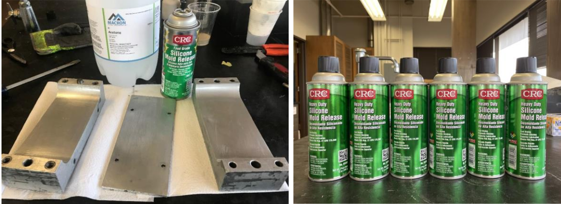
Figure 38. Aluminum mold cleaned with acetone (Reprinted from Copeland, 2020) and coated with silicone mold release spray.
