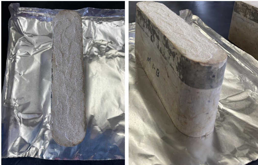
Figure 30. Aluminum foil folded on 3 sides to catch any proppant that falls off the sample.
