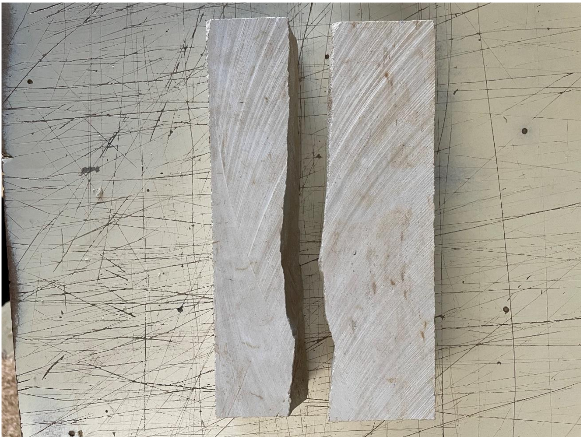
Figure 14. Fractured outcrop sample in progress.
