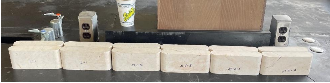
Figure 29. Six finished samples ready for fracture conductivity test preparation.
