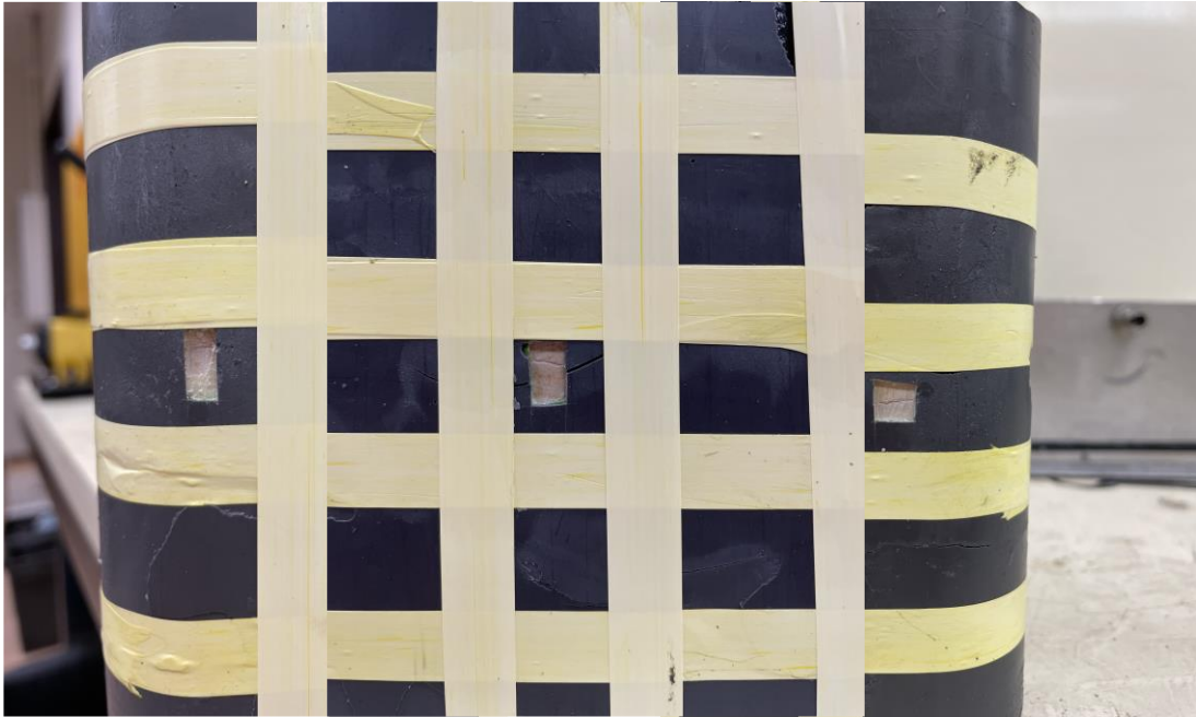
Figure 43. Three pictures put together to display the copious amount of Teflon tape applied to the sample.
