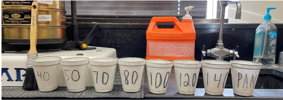
Figure 51. Cups used for proppant sieve analysis in the corresponding sieve mesh sizes used for this study: 40, 50, 70, 80, 100, 120, 140, and pan.
