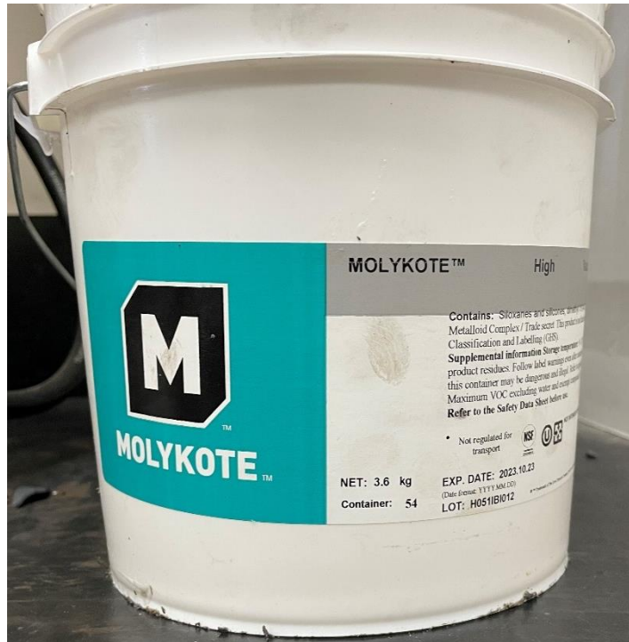
Figure 45. Molykote vacuum grease used during sample installation into the conductivity cell.
