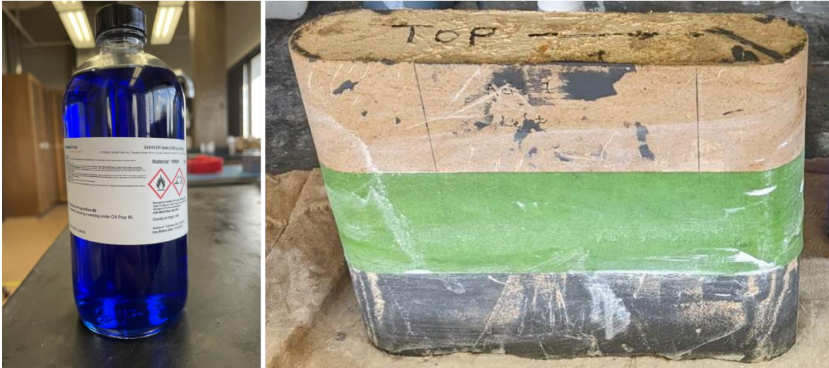
Figure 36. Left - Momentive SS4155. Right - sample with dried primer coating (Modified from Fojtasek, 2022).
