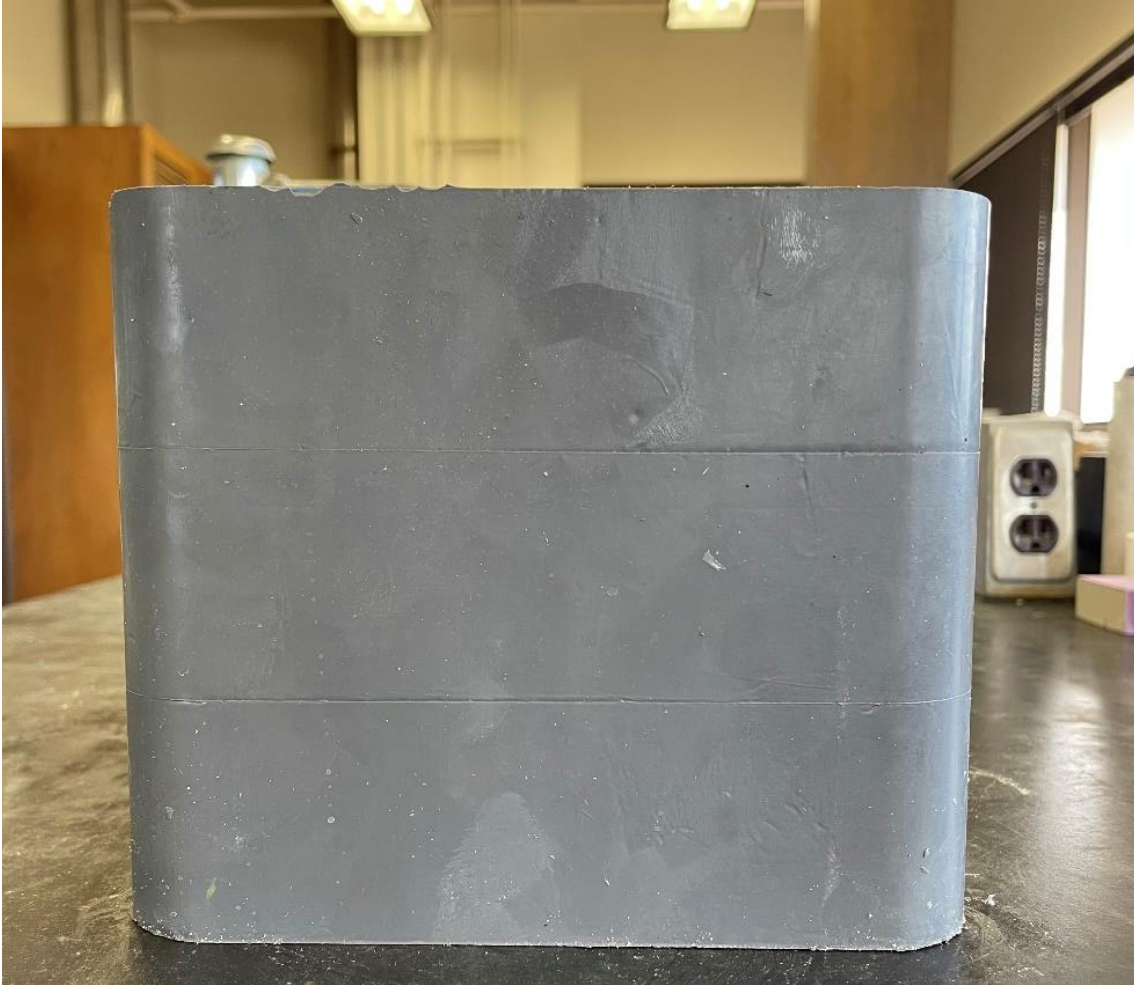
Figure 41. Completed sample preparation, ready for fracture conductivity testing.
