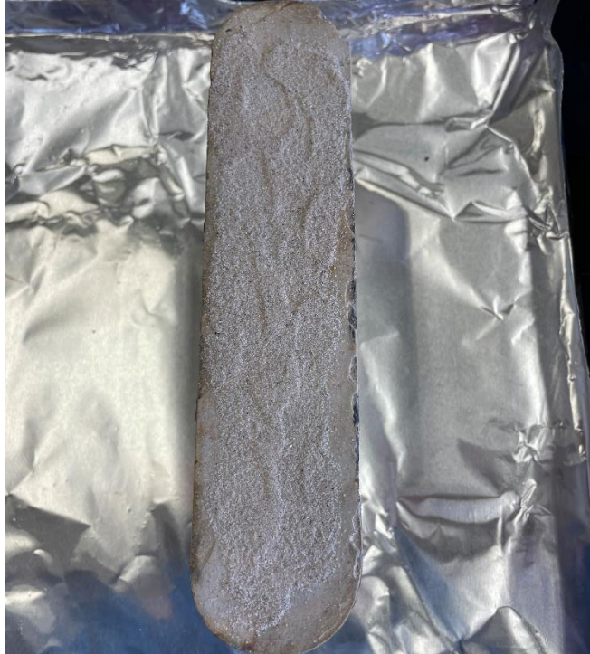
Figure 33. Sample after proppant has been poured on but before smoothing.
