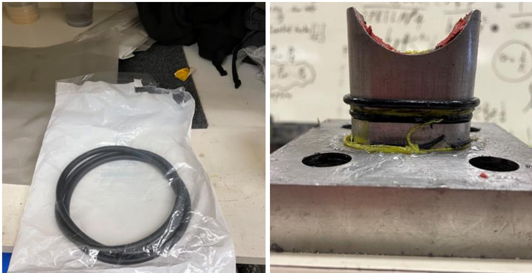
Figure 56. Left - New O-rings for the top and bottom pistons. Right - A new O-ring for a flow insert.
