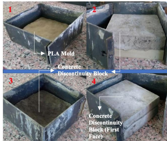
Figure 1.11: Discontinuity replication procedure (Isleyen & Duzgun, 2018).
