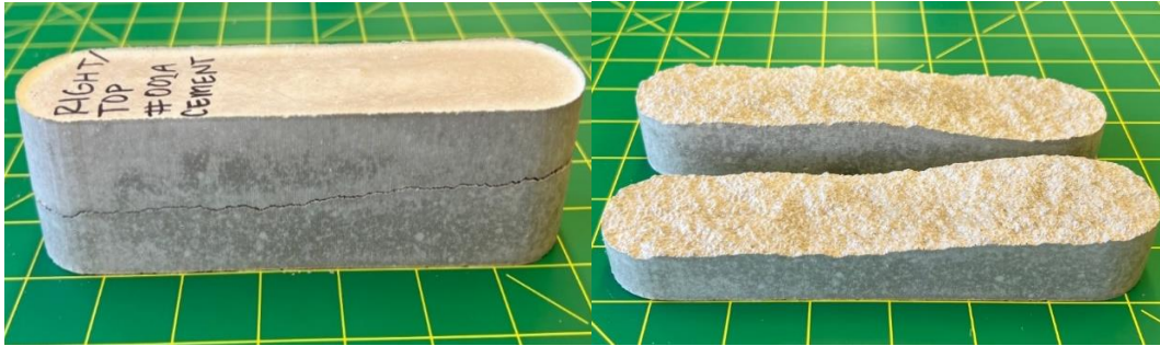
Figure 3.7 : Cement replicas cast from mold of 3D printed conductivity samples
