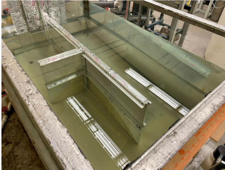
Figure 3.3 : Final Proppant Transport Apparatus
