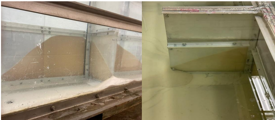
Figure 3.4 : Duning shown from Proppant Transport Experiment
