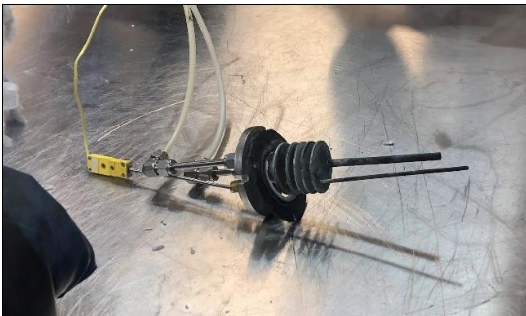
Figure 3. Tube Furnace lid with heat shield and thermocouple protrusions.
