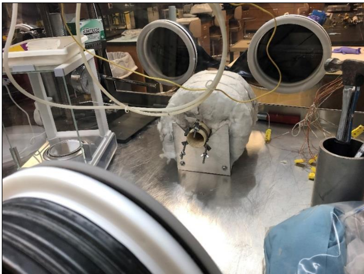
Figure 2. In-glovebox alumina tube furnace with Mettler-Toledo scale on the side.
