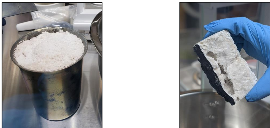
Figure 24. Salt sample produced in the large nickel crucible.
