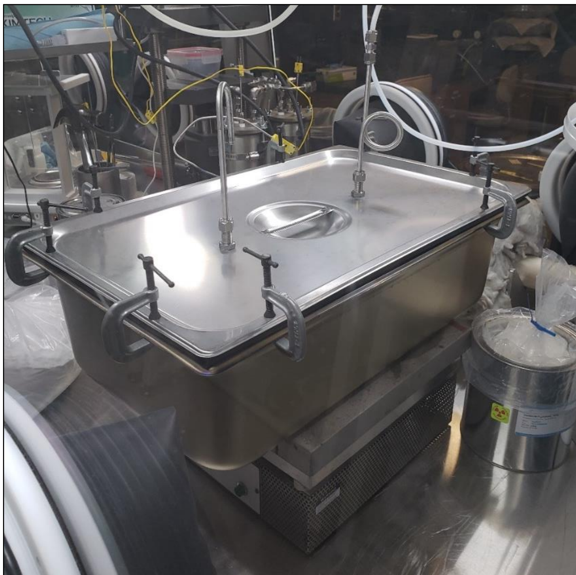
Figure 10. The purification system on top of the hot plate.
