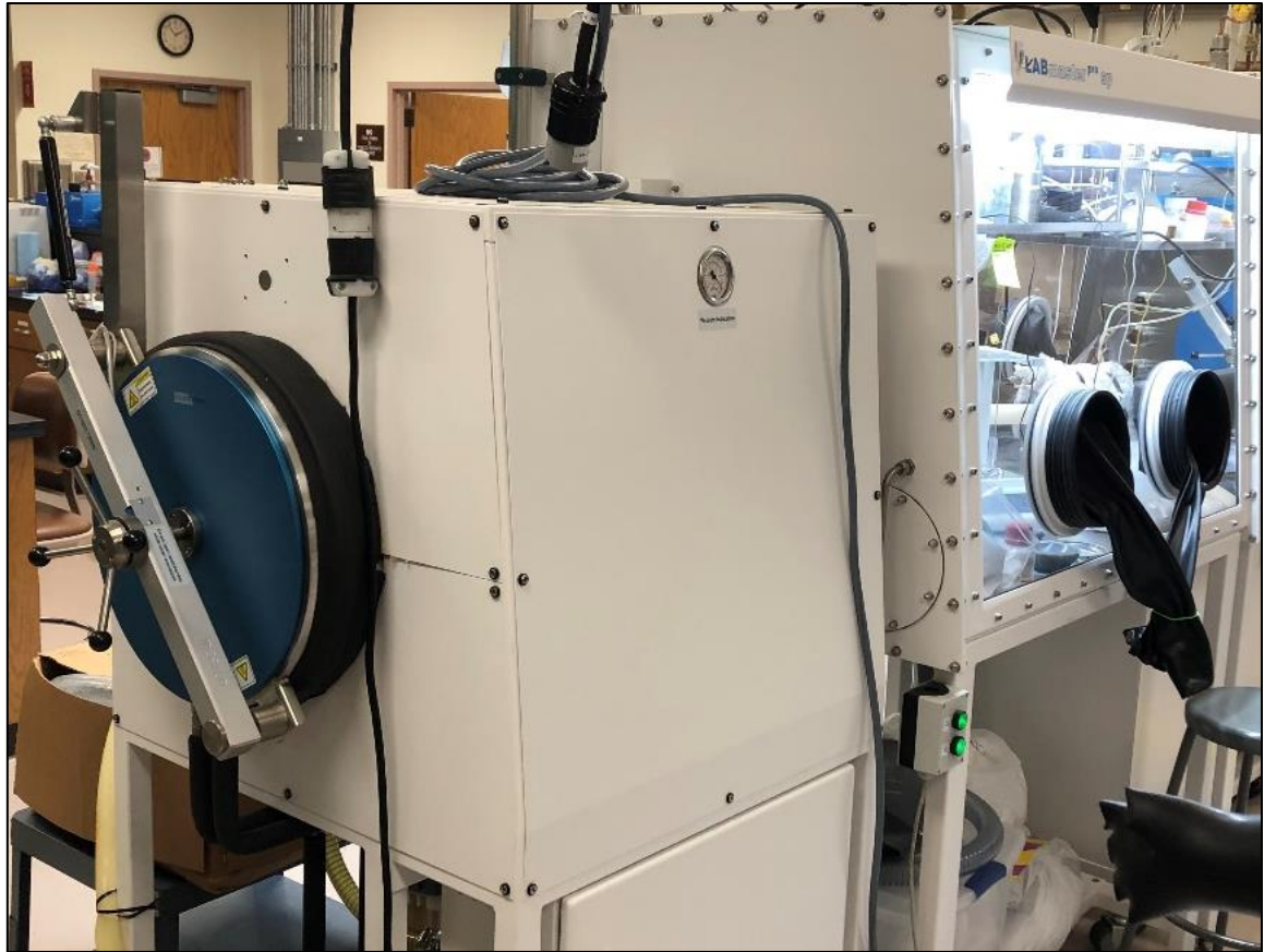
Figure 11. The BRAUN MB-VOH-600 attached vacuum furnace.
