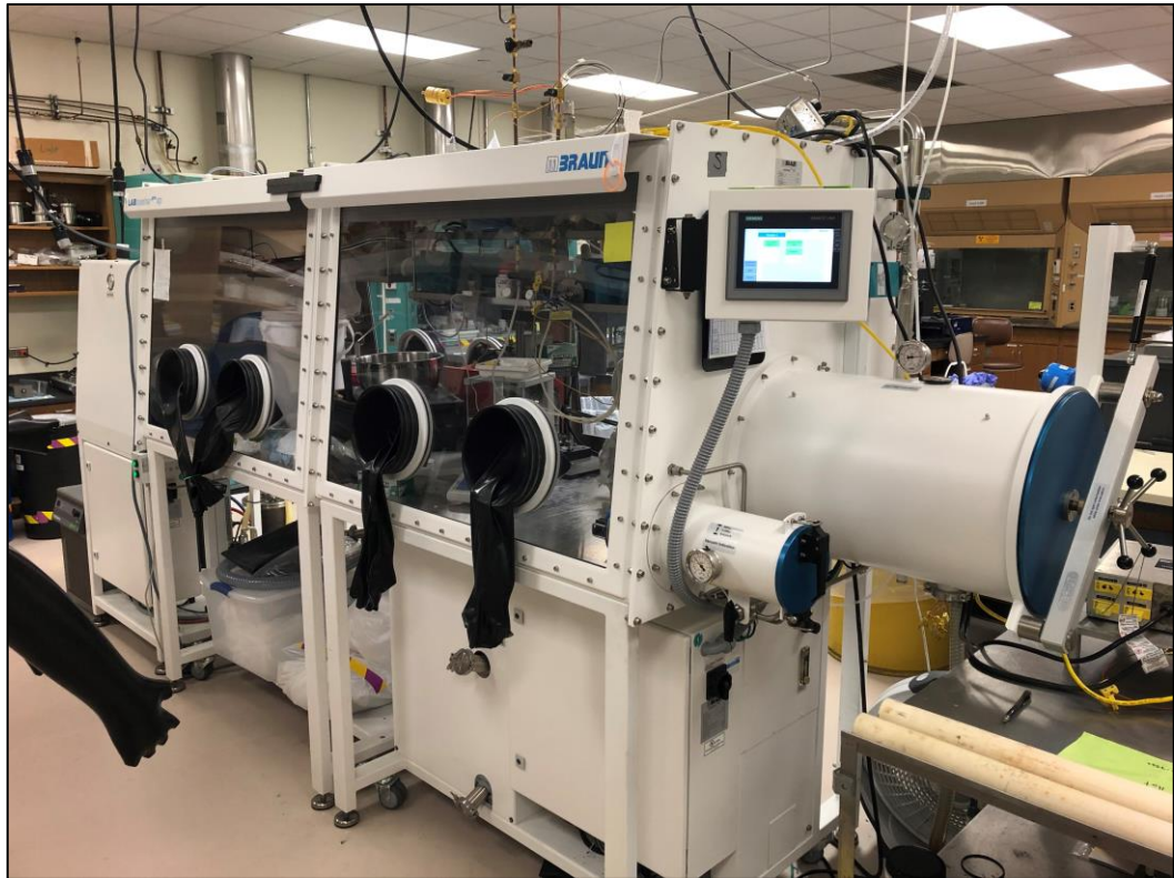
Figure 1. MBRAUN glovebox housing the salt experiments.
