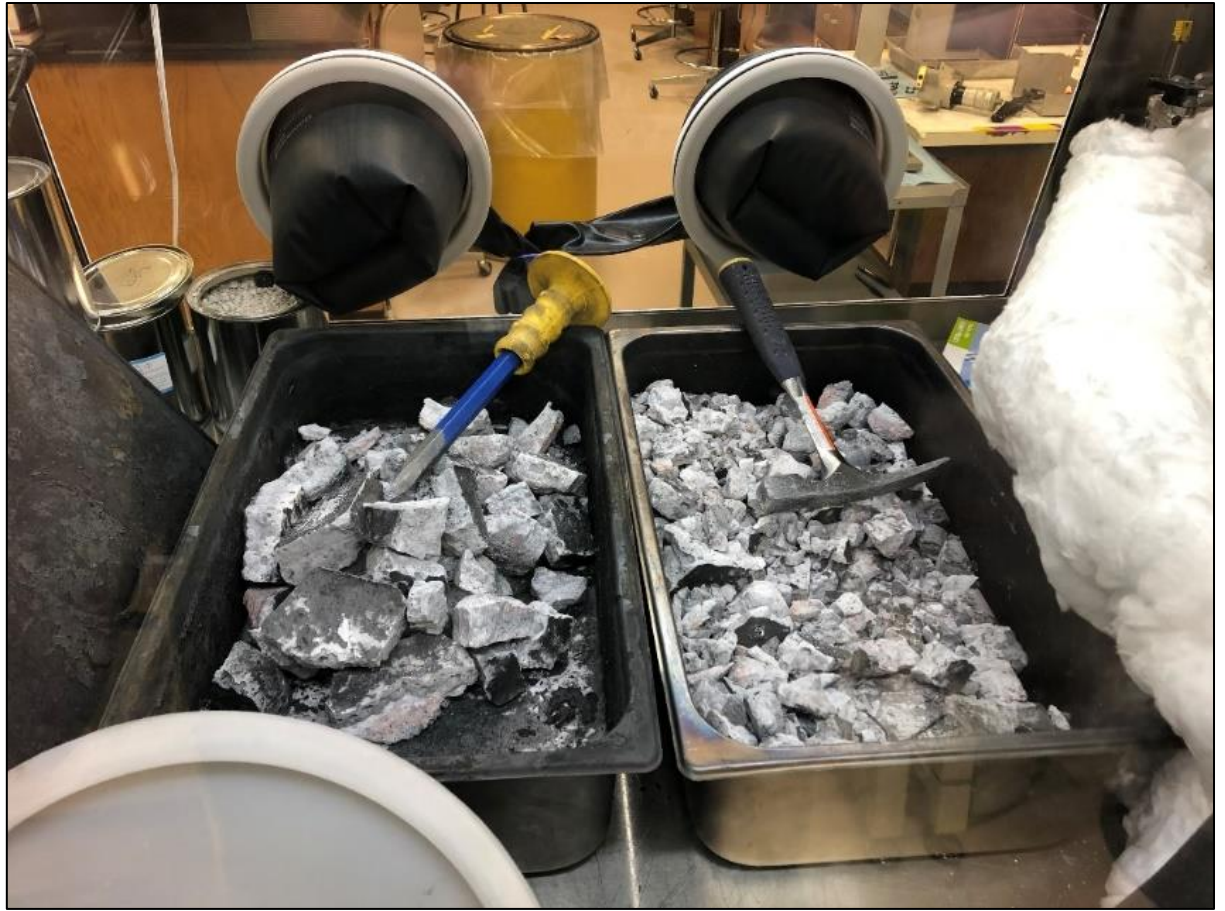
Figure 26. Salt in pans being broken up by masonry hammer and chisel.
