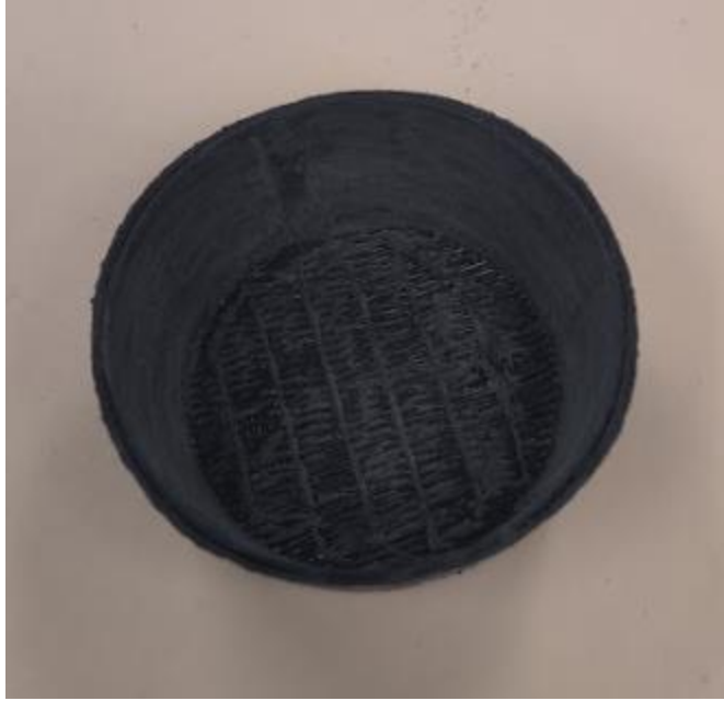
Figure 35: Interior ceiling after grinding away support structure
