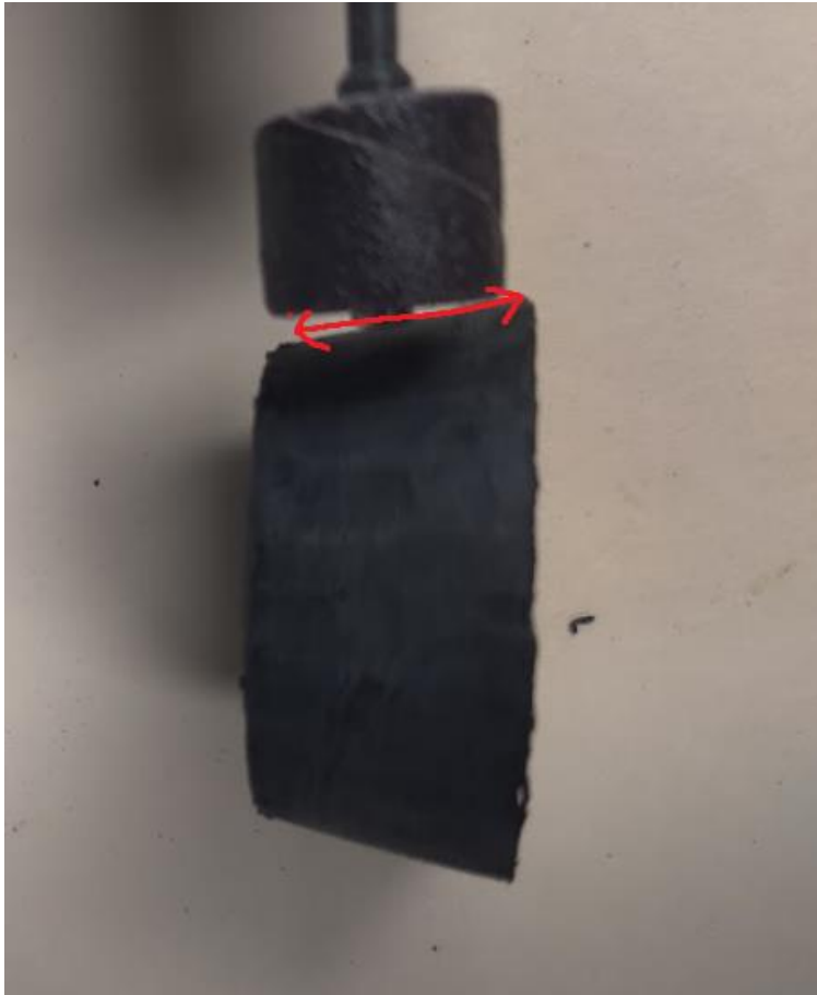
Figure 36: Sanding vertically along the taper of the part until layers are no longer visible
