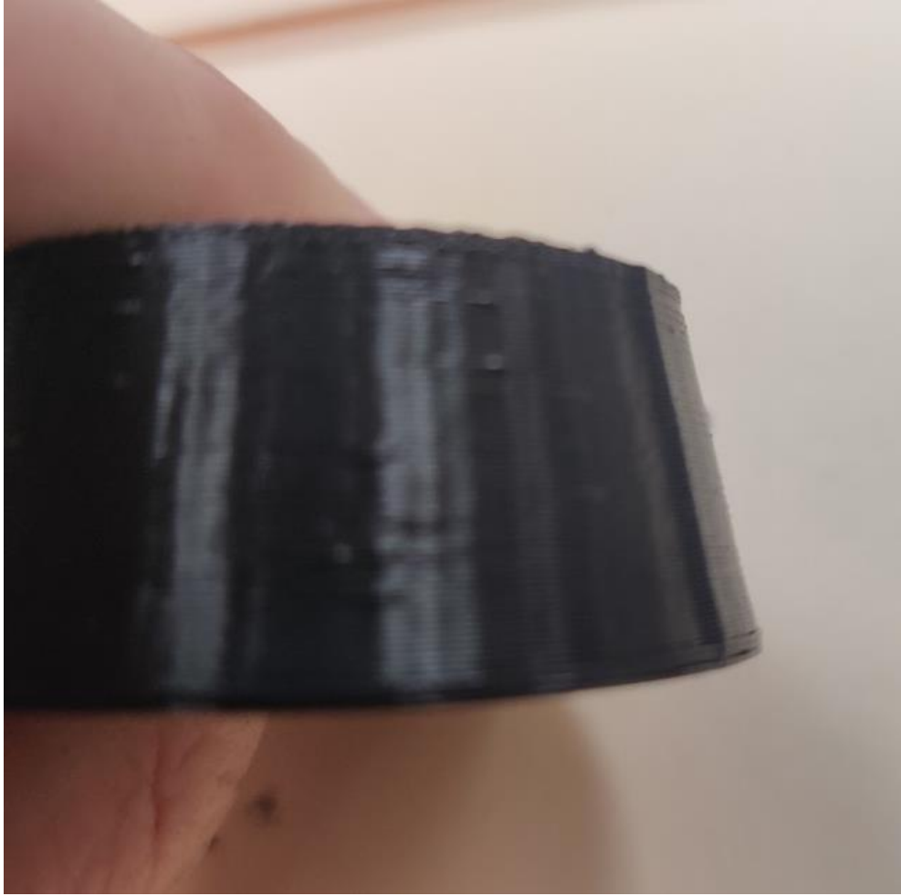
Figure 38: Buildup of filament near the build platform due to reduced print speed
