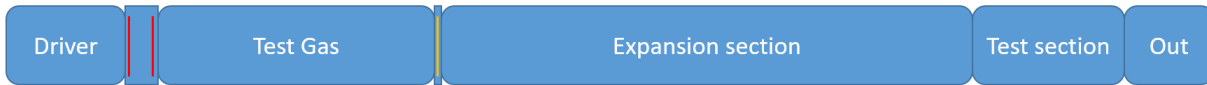
Figure 1.3: HXT Anatomy. Red lines represent metal burst discs while the orange line represents the mylar sheet
