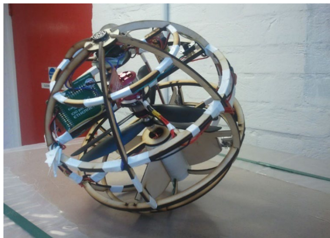
Figure 37 Example of a flying Spherical Robot
