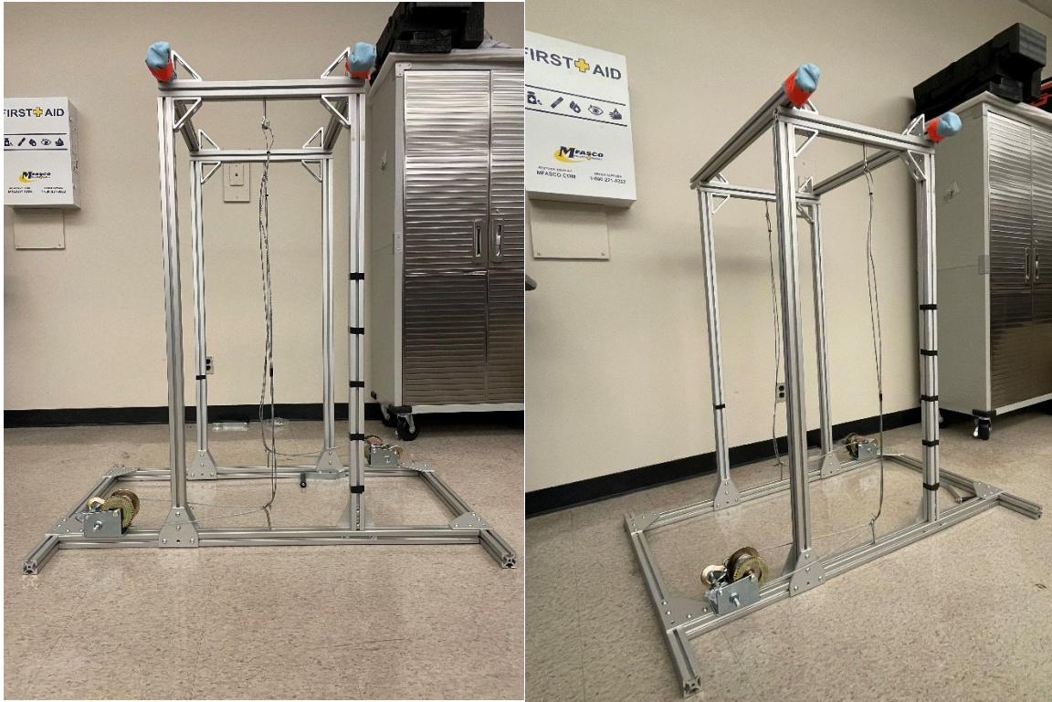
Figure 74 Test stand for collecting Bouncing Data
