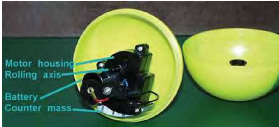
Figure 16 ‘Squiggleball’ opened to show the interior parts
