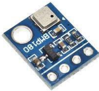
Figure 69 BMP 180 Pressure Sensor
