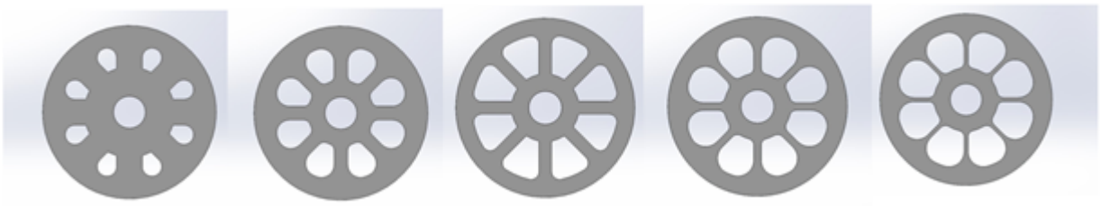
Figure 3.5: Example of cutout geometry
