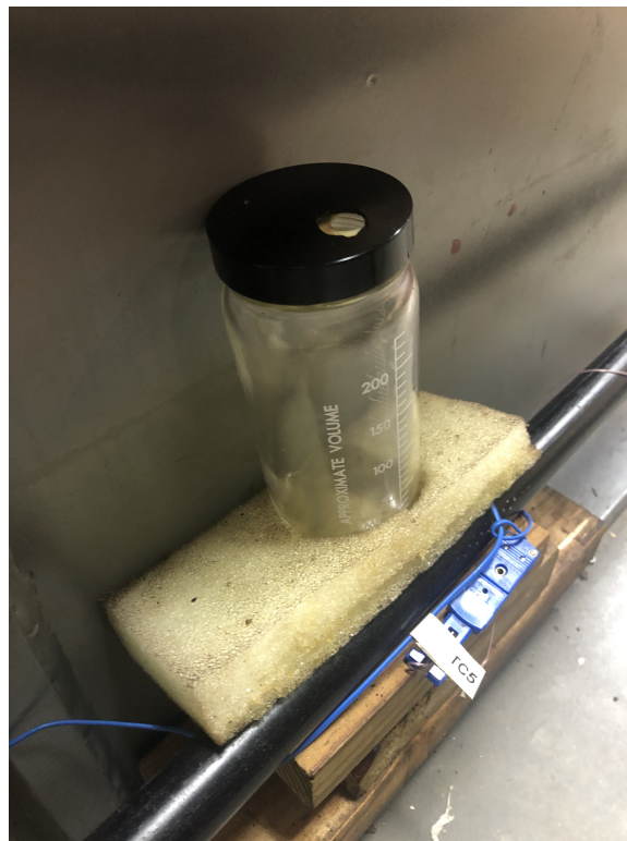
Figure 3.13: Leakage collection container
