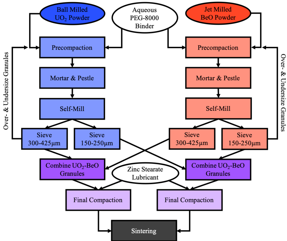
Figure 3.1 Pellet fabrication flow chart for dispersed \text{UO}_2\text{-BeO} composite compacts with two parallel granulation steps for \text{UO}_2 (blue) and \text{BeO} (red) prior to final compaction (purple) and sintering (gray)
