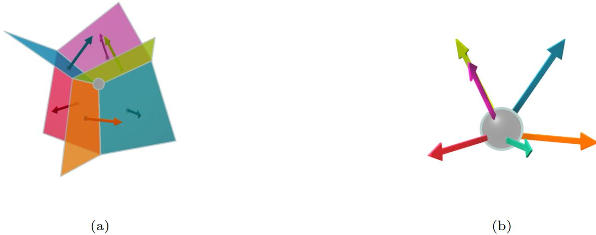
Figure 2.1: (a) A three-dimensional view of the possible micro cracks or fracture microplanes intersecting at a material point, (it shows only six microplanes but many more can be accommodated) and (b) the corresponding normal directions to the fracture microplane surfaces at the material point.
