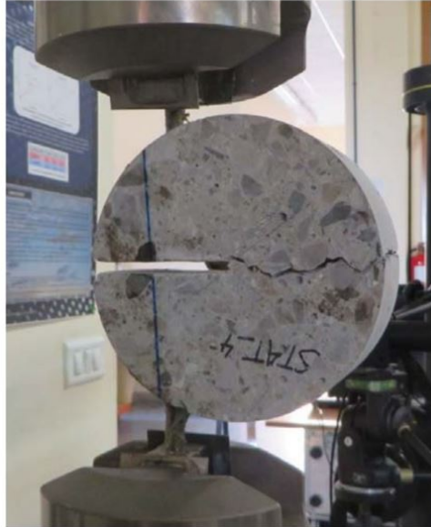
Figure 1.11: Crack propagation for a compact tension test from Fernández-Canteli et al. [19].
