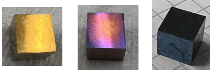
Figure 27. Color of heat-treated cubes at 425°C for 15, 30 and 50 minutes
