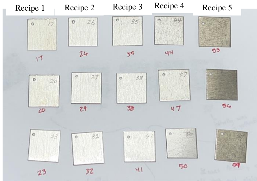
Figure 19. Nickle plated nickel squares before heat treatment
