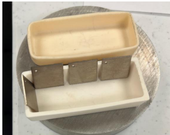
Figure 14. Ceramic boat for quartz tube furnace
