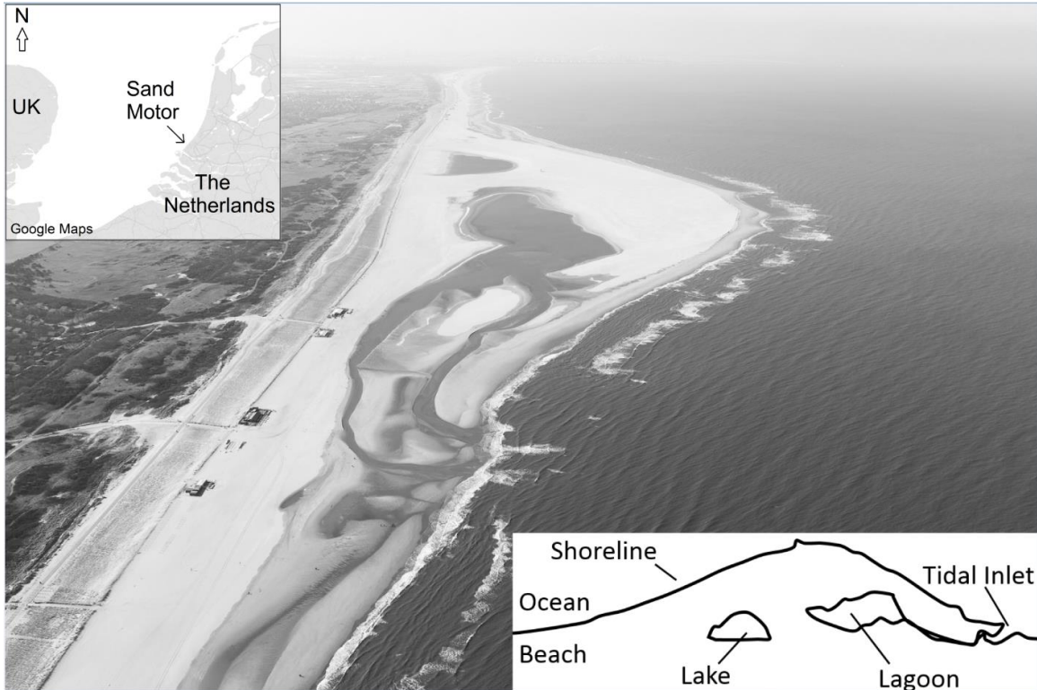
Figure 3.3. Aerial photo of the Sand Engine dated March 28, 2013. The coastline profile seen here is very similar to the one used as the initial coastline in the first project (March 1, 2013). The tidal inlet, lagoon, and lake are neglected in model simulations. Photo courtesy of the Dutch Ministry of Infrastructure and the Environment. The top left map insert is courtesy of Google Maps.
