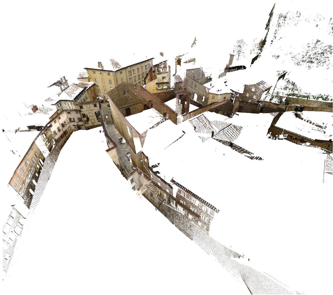
Figure 12 Colorized laser scan point cloud of Chiesa di Sant'Agostino in Castiglion Fiorentino, Italy. Laser scan by Mark Gastelo, Bob Warden, and the author; image created by the author.
