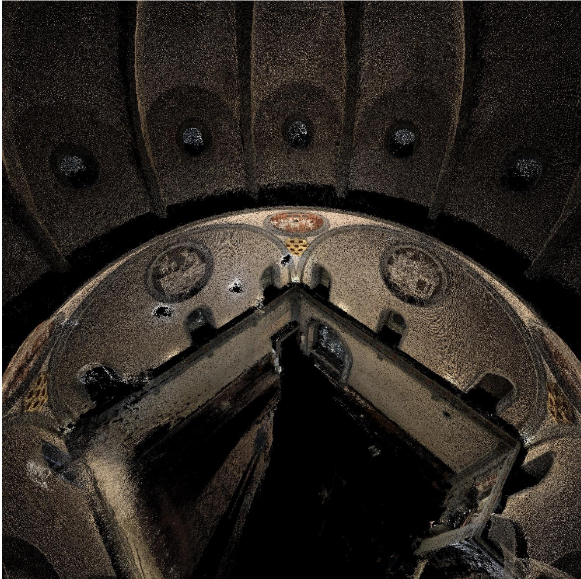
Figure 2 Colorized photogrammetry point cloud of the interior of the Sacristy of Basilica di San Lorenzo in Florence, Italy. This is an example of Saunders' 'verduta per angelo' created by the author.
