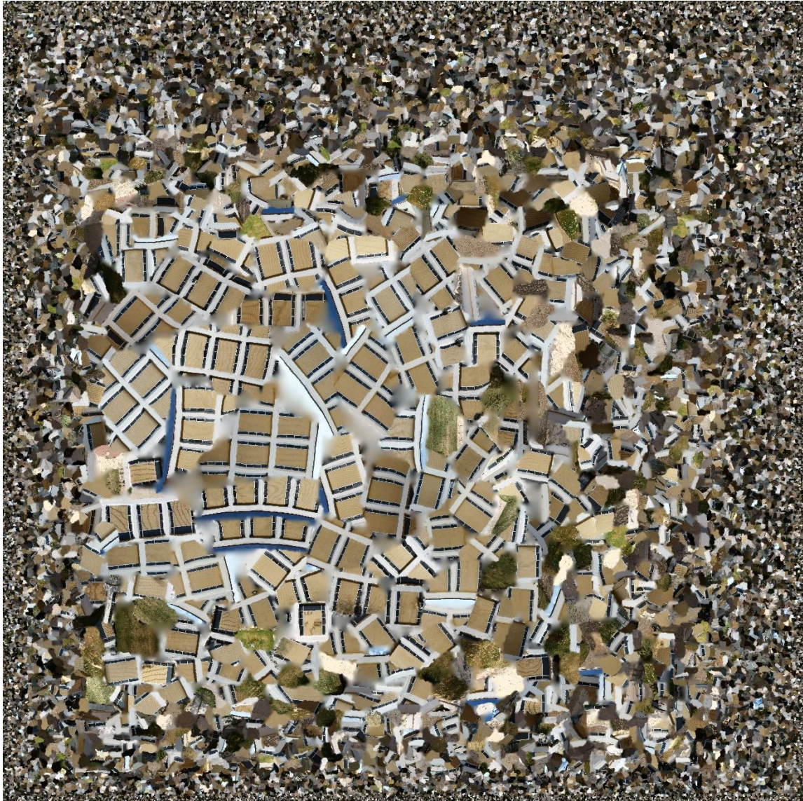
Figure 32 Texture image, generic mapping with mosaic blending, from surface model (.obj) export out of Agisoft Metashape - textured photogrammetry surface model created by the author of Biological Sciences Building - West, Texas A&M University, College Station, Texas, United States.
