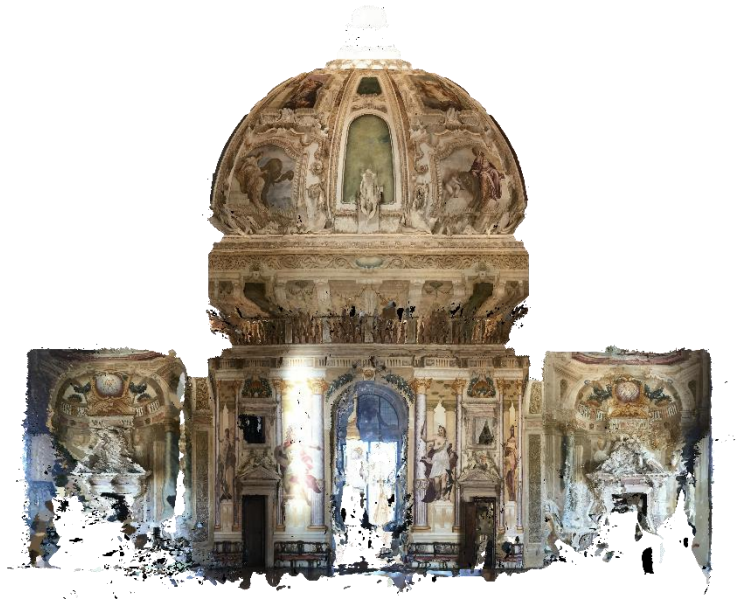
Figure 29 Textured photogrammetry surface model of the interior of Villa La Rotonda, Vicenza, Italy. Photogrammetry and imaging by the author.
