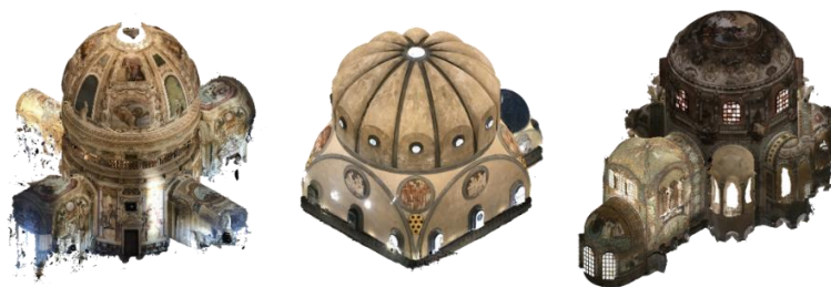
Figure 14 Textured photogrammetry surface models created by the author using an iPhone 7 and Agisoft Metashape: (from left to right) Villa La Rotonda, Vicenza, Italy; Sacristy of San Lorenzo, Florence, Italy; Basilica di San Vitale, Ravenna, Italy.
