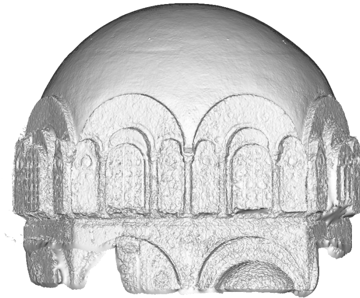
Figure 23 Monochrome photogrammetry surface model of the interior of Battistero Neoniano, Ravenna, Italy. Photogrammetry and imaging by the author.
