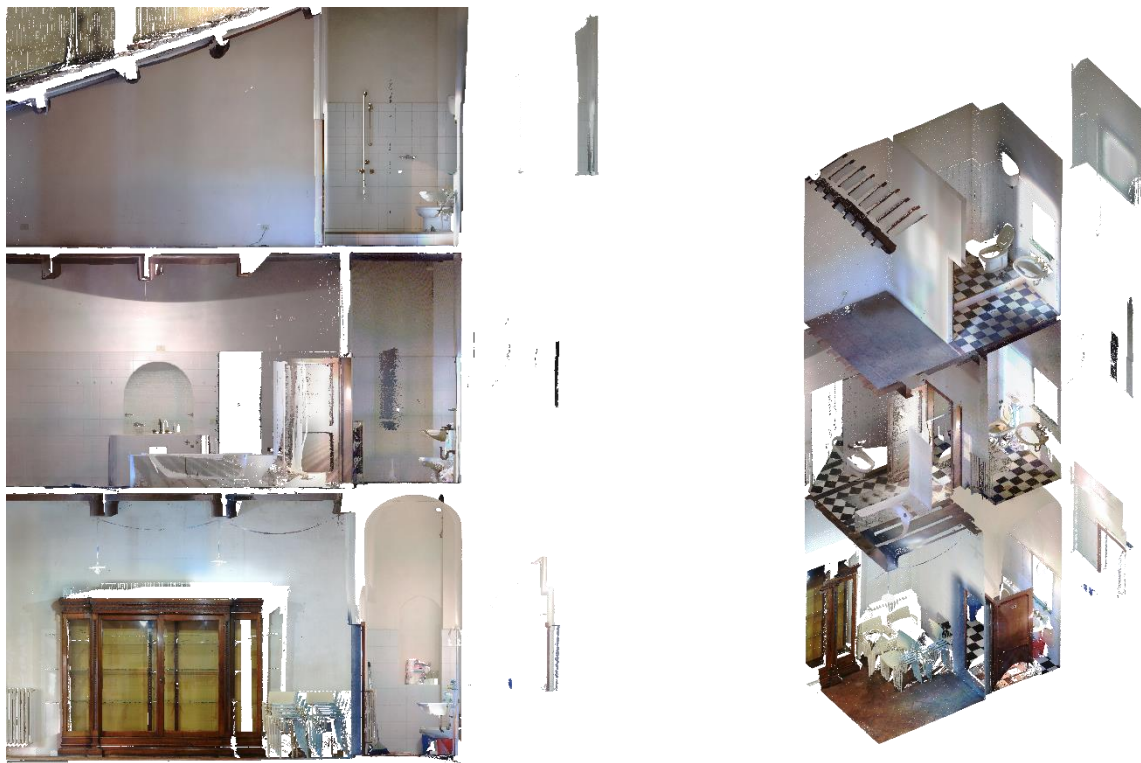
Figure 26 Mirror Reflection Error / Noise - colored laser scan point cloud of the interior of Palazzo Gaci in Castiglion Fiorentino. Laser scan by Mailee Shaw, Ashlon Richburg, Bob Warden, and the author; imaging by the author.
