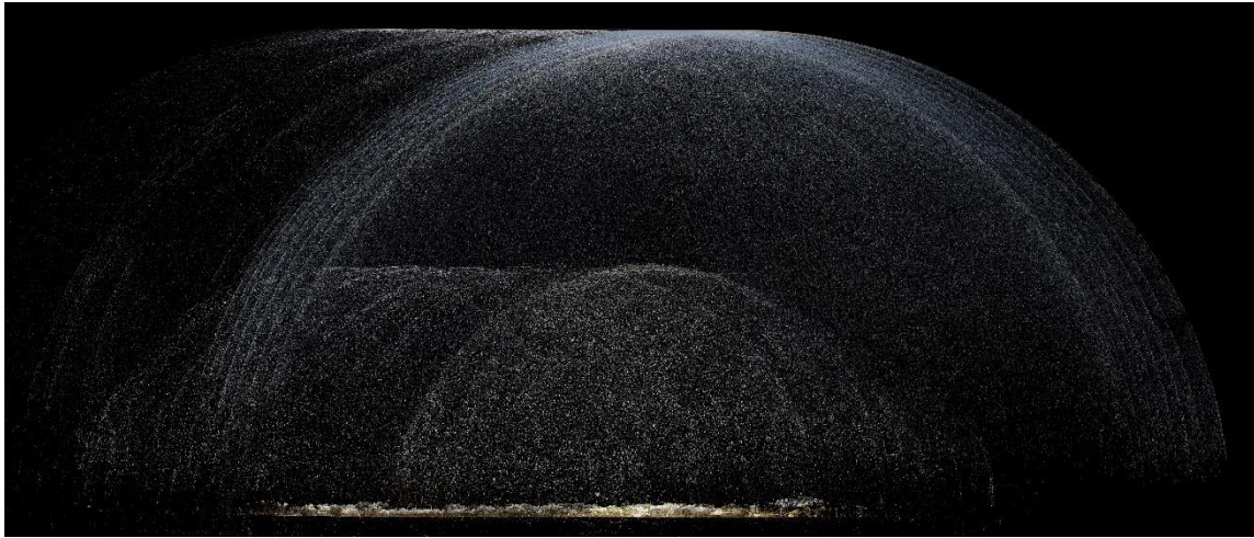
Figure 52 Halo / dome error – colorized laser scan point cloud of Buffalo Gap, Texas, United States. Project led by Greg Luhan and the Department of Architecture, Texas A&M University, lasering scanning and imaging by the author.
