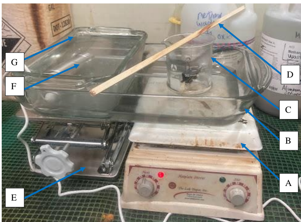
Figure 8. Chemical Etching Setup. Where, A: Hot Plate, B: Glass Pan, C: 250 mL Beaker, D: Tool Hanger, E: Jack Plate, F: Ultrasonic Pulser, G: Chilled Bath
