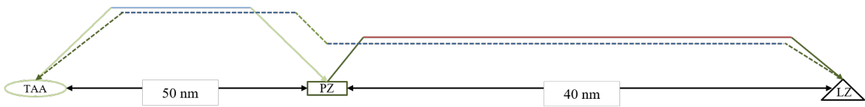
Figure 5.4: A proposed 14-stage mission with five mission stage types. The mission starts and ends at the Terminal Arrival Area (TAA).
