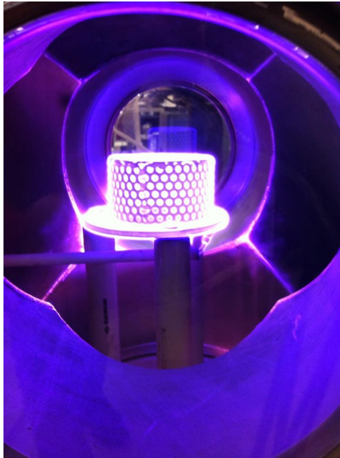
Figure 3.8: First nitriding cage setup.
