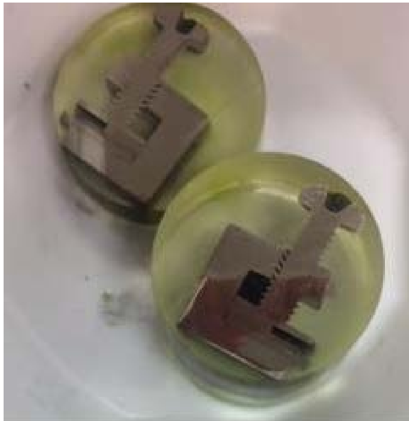
Figure 10.2: The image of a diffusion couple after being cut by half.
