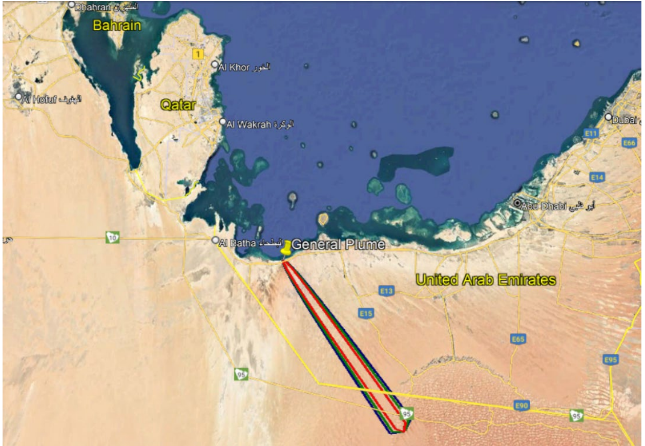
Fig 14. Plume dispersion for 10% source term activity released before cooling (fuel burnup step 32) for most probable scenario with atmospheric stability class, D.
