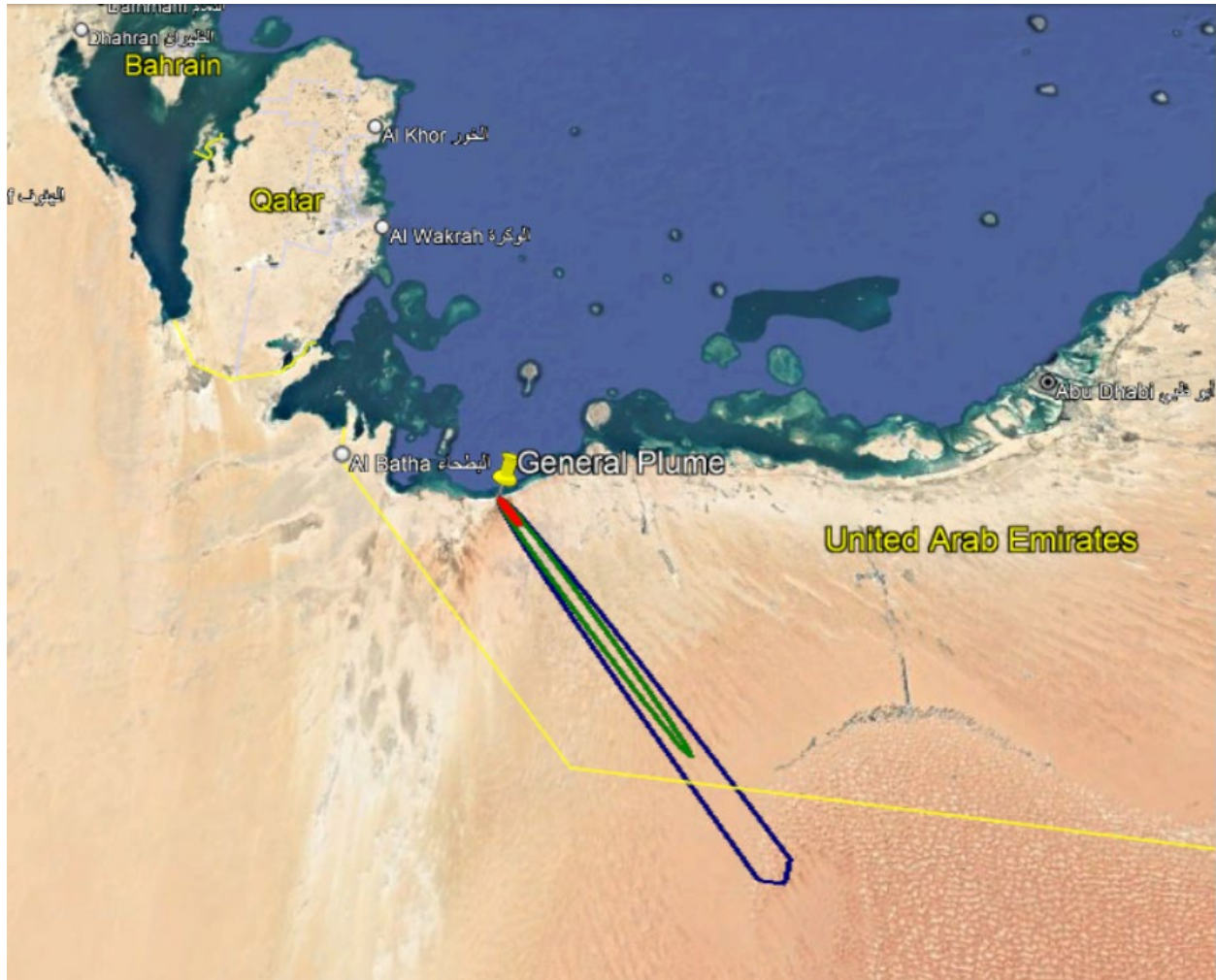
Fig 20. Plume dispersion for 1% source term activity released before cooling (Fuel burnup step 32) for most probable scenario with atmospheric stability class, D.
