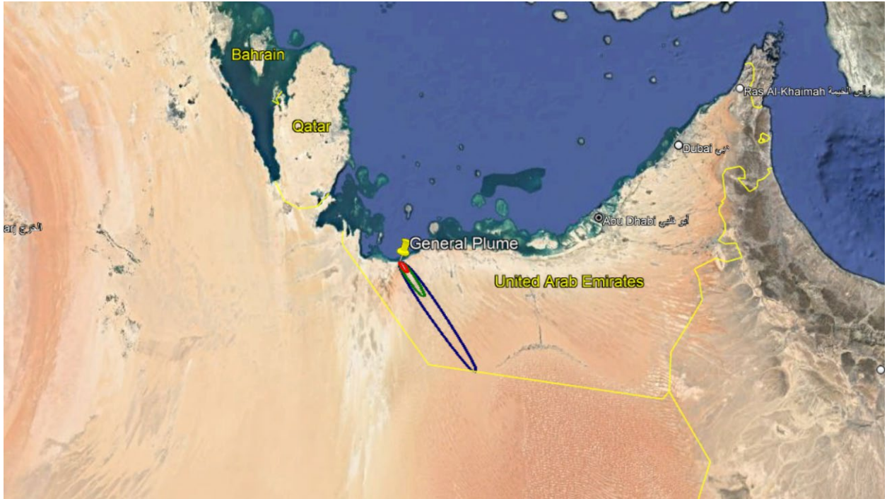
Fig 15. Plume dispersion for 10% source term activity released after one year cooling (Fuel burnup step 35) for most probable scenario with atmospheric stability class, A.
