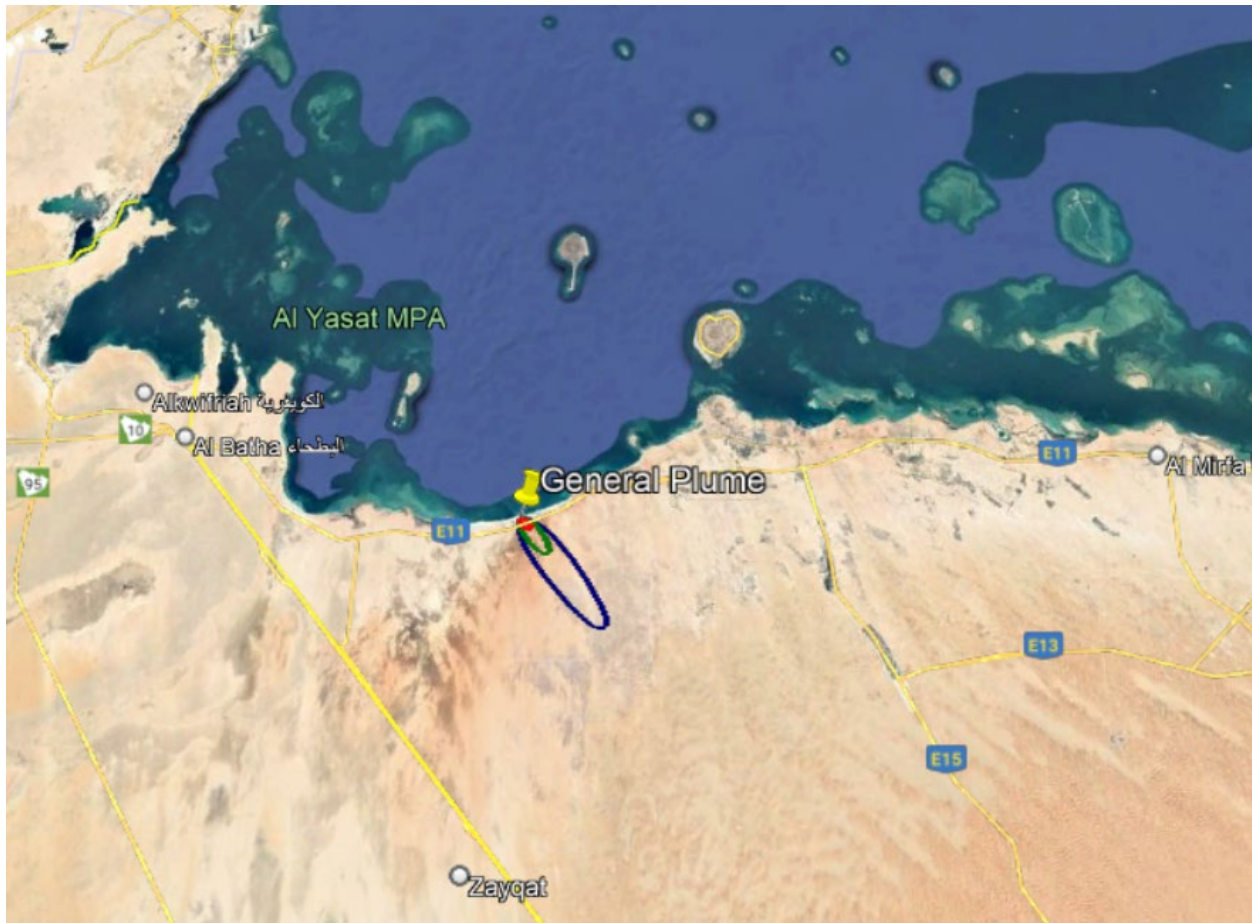
Fig 18. Plume dispersion for 1% source term activity released before cooling (Fuel burnup step 32) for most probable scenario with atmospheric stability class, A.
