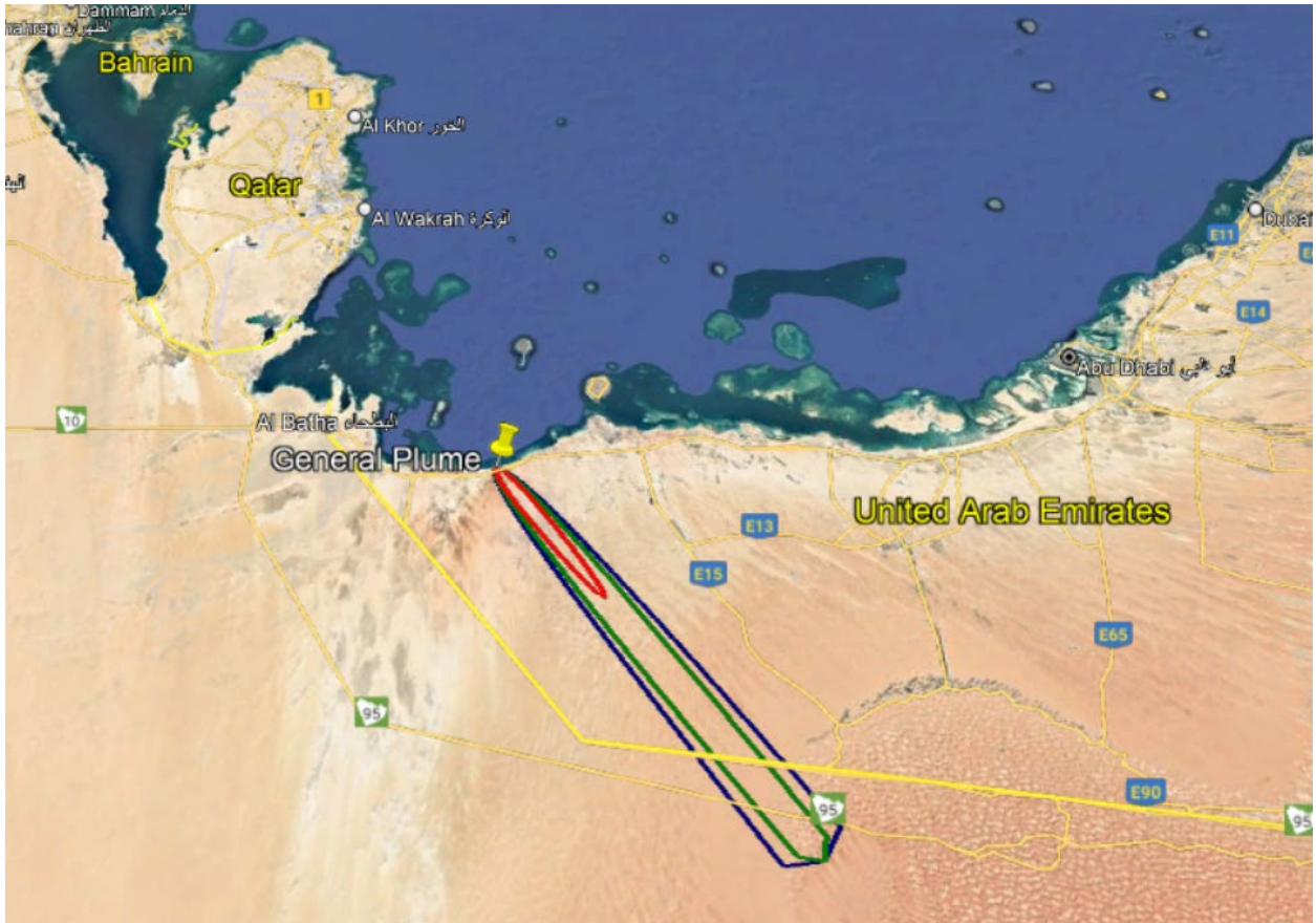
Fig 13. Plume dispersion for 10% source term activity released before cooling (fuel burnup step 32) for most probable scenario with atmospheric stability class, C.
