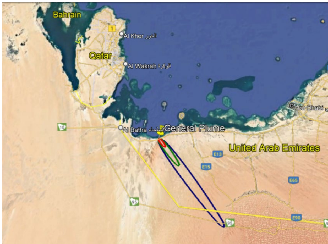
Fig 12. Plume dispersion for 10% source term activity released before cooling (Fuel burnup step 32) for most probable scenario with atmospheric stability class, A
