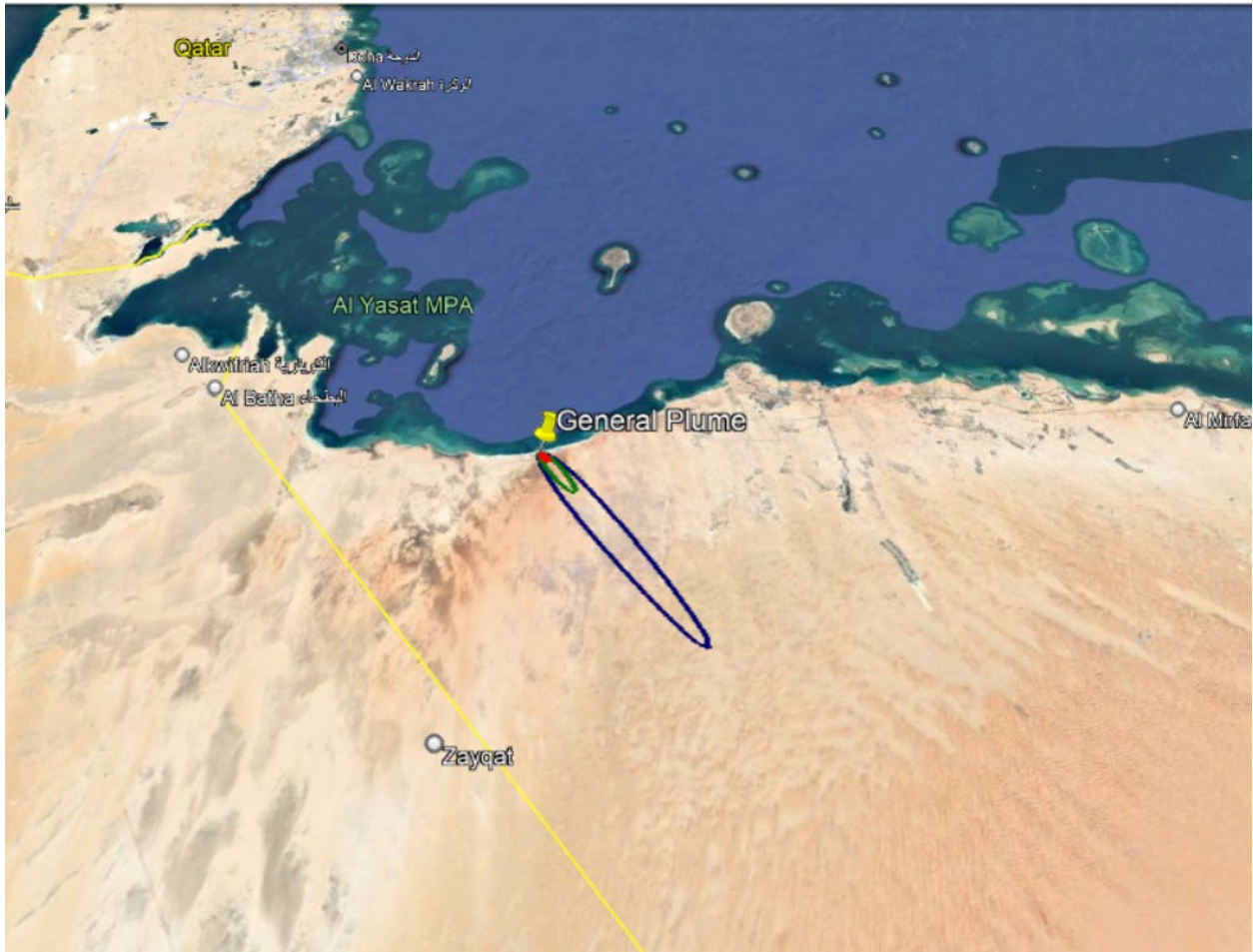
Fig 22. Plume dispersion for 1% source term activity released after one year cooling (Fuel burnup step 35) for most probable scenario with atmospheric stability class, C.
