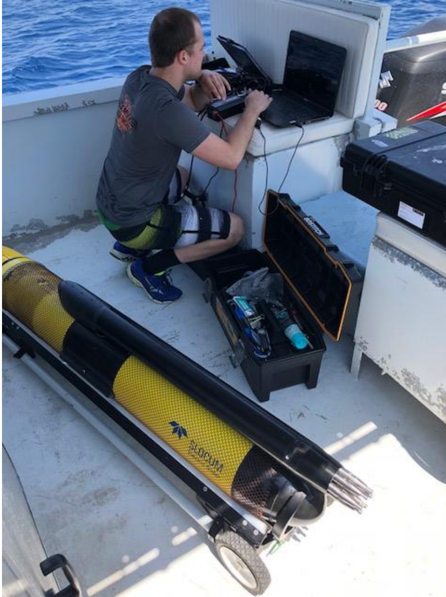
Figure 1.2: Graduate student Christian Nygren deploying Slocum glider (Sverdrup) to study turbulence on the continental slope of Gulf of Mexico. Picture source: GERG Facebook page.
