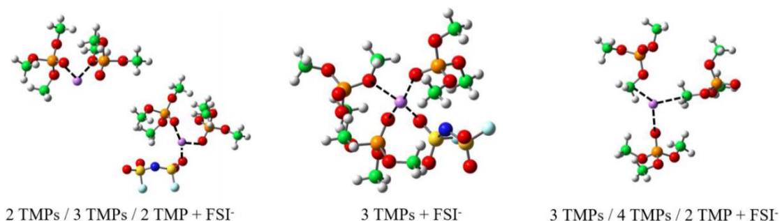
Figure 3.2 Solvation structures are identified, left: TMP 2 /TMP 3 /TMP 2 + FSI - , center: TMP 3 + FSI - and right: TMP 3 /TMP 4 /TMP 2 + FSI - . Li (violet), N (blue), C (green), P (orange), H (white), F (cyan), S (yellow), and O (red).
