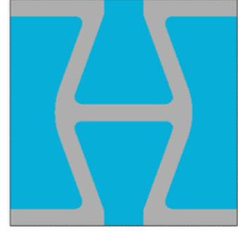
(c) Reentrant substructure geometry.
