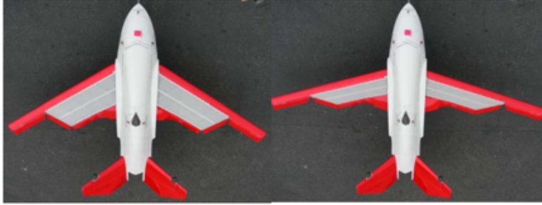
Figure 1.1: The sweep morphing wing used as a case study in this work. Reprinted from [21].
