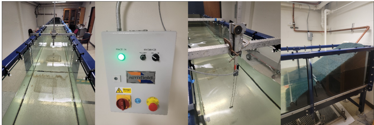
Figure 3.1: From the left: first image showing the top view of the tank; second image showing the wave maker controller; third image showing closer view of the wave gauge with tapes and foam stripes to fix the wires from the gauge to reduce vibrations; fourth image showing the prism shape permeable beach accounting for wave absorption at far end of the tank
