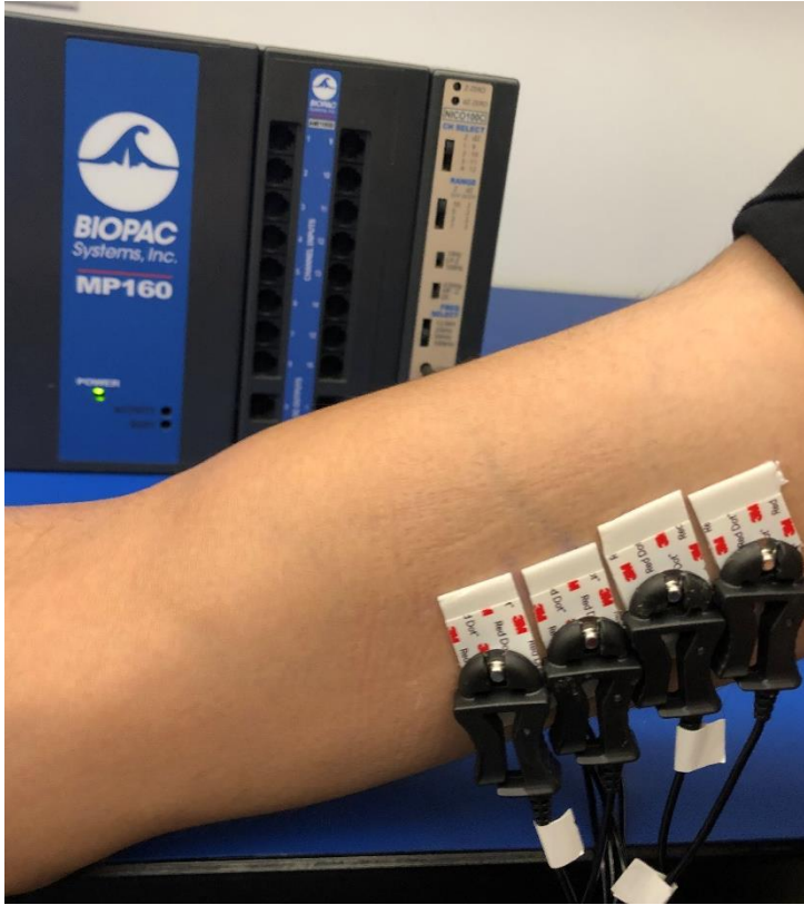
Figure 5.3. Electrode location in left upper arm
