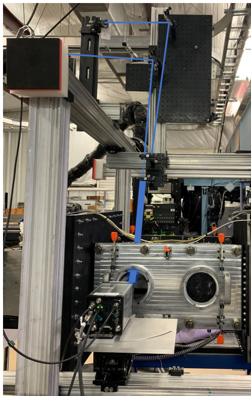
Figure 6.12: PLIF thermometry setup. Only one beam shown beyond focusing optic for clarity.
