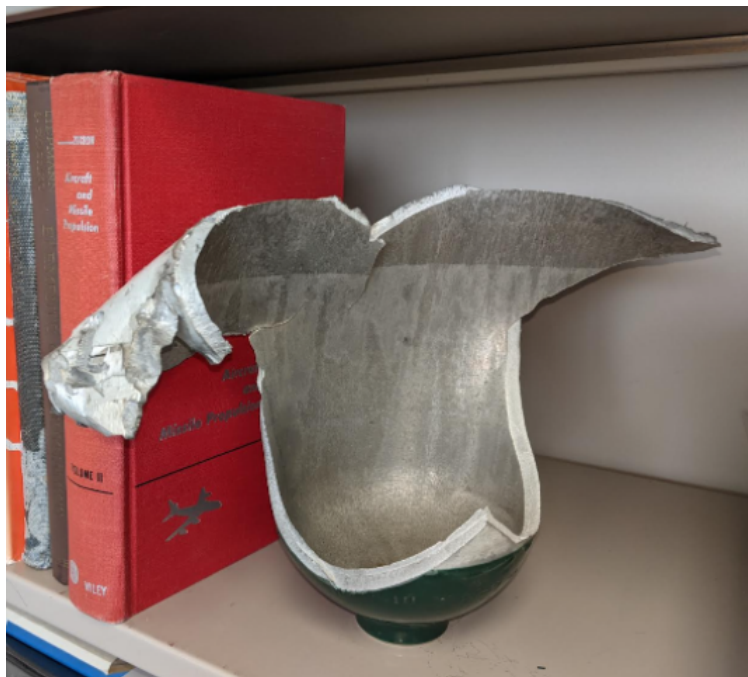
Figure 16: Aero 402 Nitrous Oxide Tank Explosion
