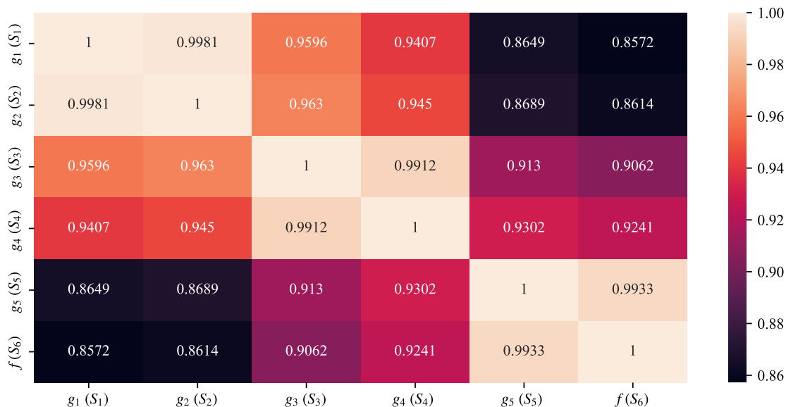
Figure 4.3: Pearson’s correlation of the RP values either computed via the high-fidelity DFT model f or predicted surrogate models g_i , i = 1, 2, \dots, 5 . As we used more descriptors, the correlation of the RP predicted via the surrogate models in comparison to the high-fidelity DFT model increased as we expected. Note that the predicted descriptors via the sub-surrogate model helped improve the regression performance.
