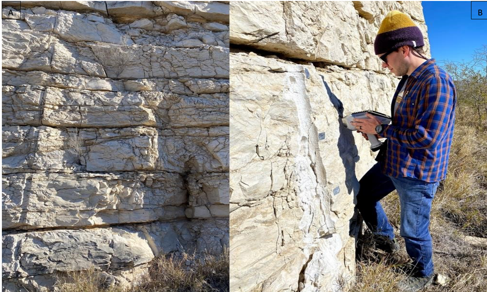
Figure 4: A (label as A and B): Austin Chalk outcrop, located along Highway 90 4.5 miles (7.2 kilometers) west of Langtry, TX showing alternating marls and highly fractured massive sections of chalk. B: Scott Gifford gathering data with the Bruker 5i XRF unit against a cleaned, buffed, flat section of the outcrop. The silver duct tape marks the approximate locations of samples every 30 cm.
