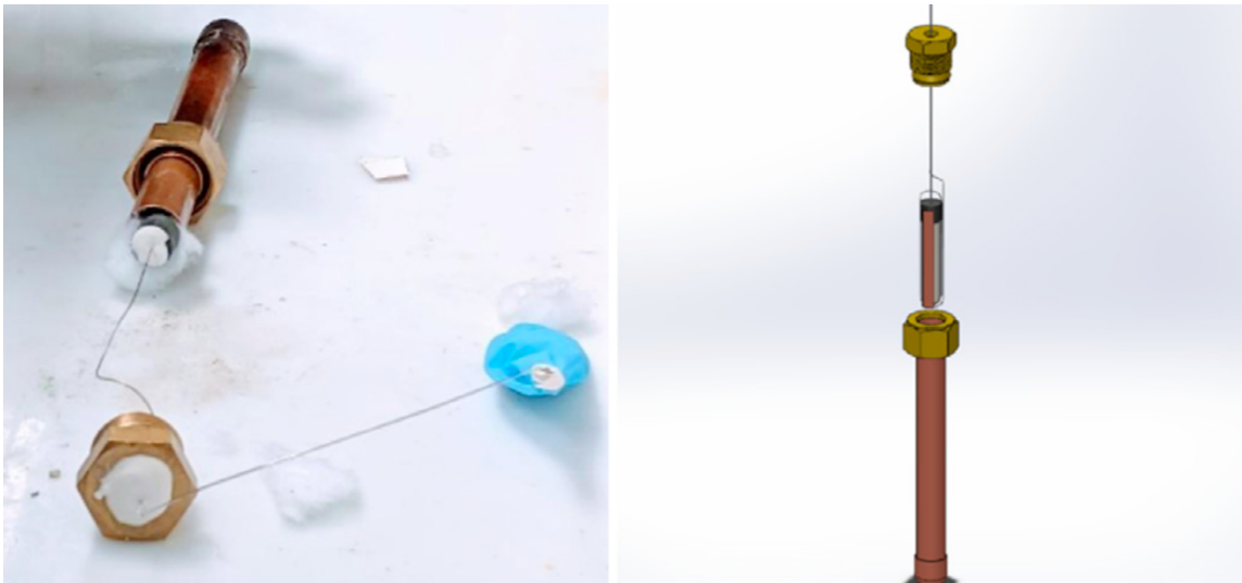
Figure 14 (left) Insertion of insulation and pellet U6-71B attached to the thermocouple into the capsule. (right) Solidworks rendering of the placement of the pellet in the capsule [19].
