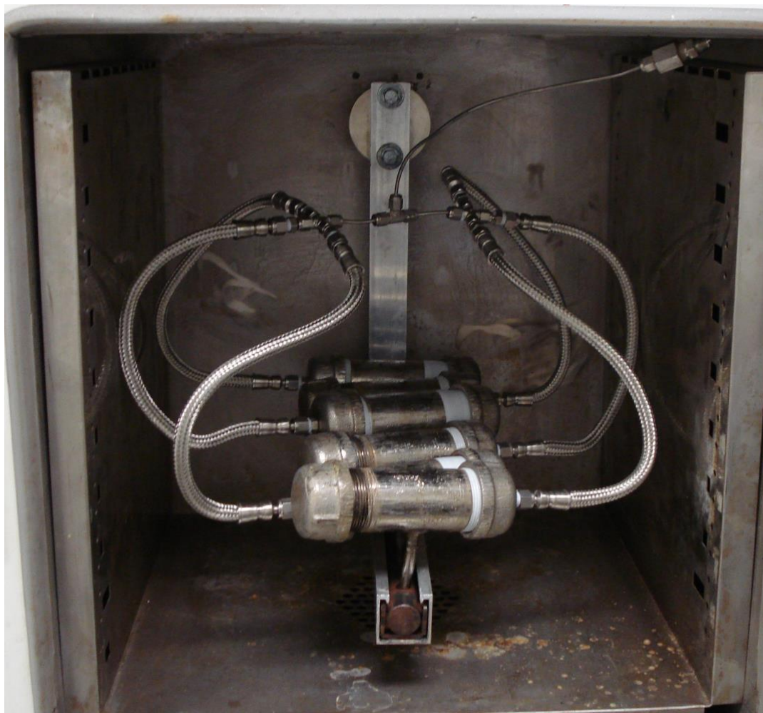
Figure 2-2. Stainless steel pipe reactor attached to swing arm in a temperature-controlled oven.
