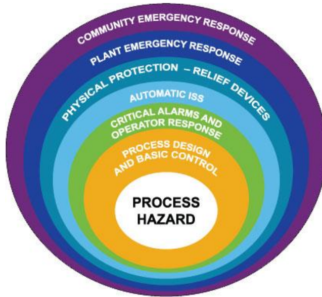
Figure 4: Sample LOPA diagram (Reprinted from [6]. Willey, R. J., 2014.)
