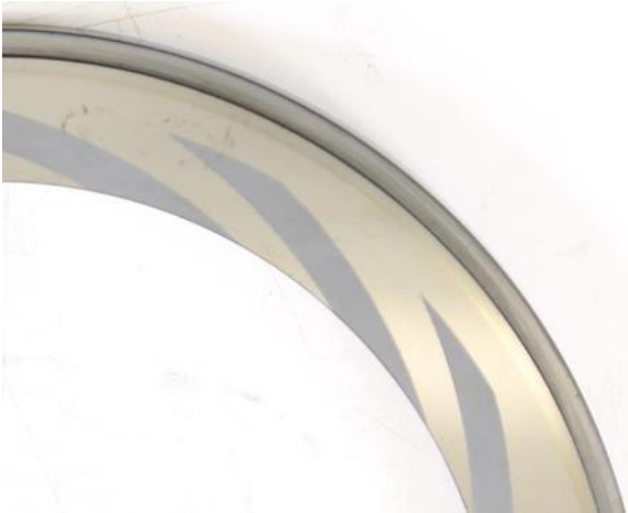
Figure 12: Typical Post-Test Condition of Stationary Spiral Groove Seal Mating Ring
