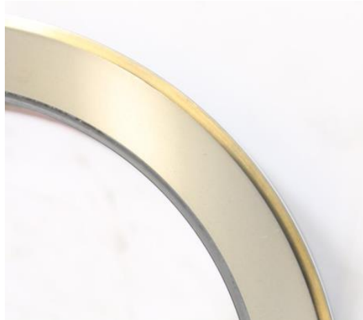
Figure 13: Typical Post-Test Condition of Rotating Seal Ring Assembly
