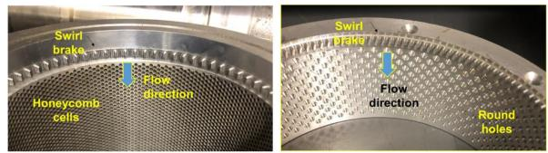
Figure 5 Photographs of a honeycomb seal and a hole-pattern seal, both with swirl brakes upstream of the seal entrance.
