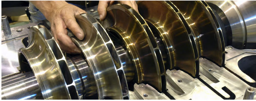
Figure 12: Picture of centrifugal compressor rotor
