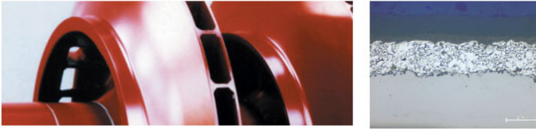
Figure 14: Picture of a coated centrifugal compressor rotor (left) and a photomicrograph of the coating layers (right)
