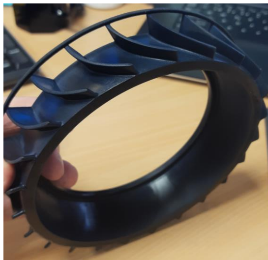
Figure 5. HAVR Helico-Axial 3D-Printed Diffuser Hub Structure with Vanes. The Diffuser was Manually Sanded to Reduce the Surface Roughness.
