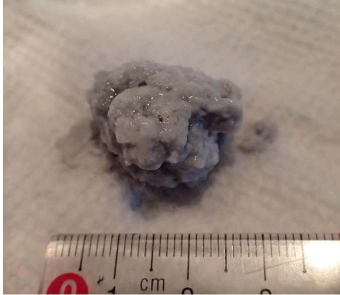
Figure 31 Mg-FD sample after 3 hours of soaking in 0.3% KCl + 0.5 gpt of PAA solution
