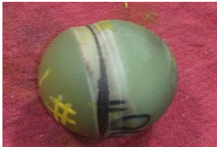
Figure 51 Example of ball deformation or egging during laboratory testing of a composite ball (Reprinted from Baihly et al., 2012)
