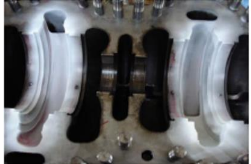
The volute was bored using boring machine and Die Penetration Tested - Result Acceptable
