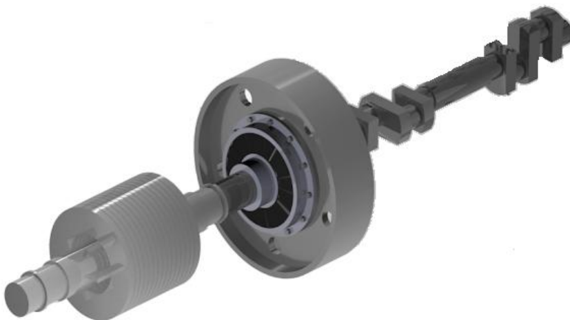
Figure 2: Schematic diagram of motor-driven Compressor drivetrain coupled with soft elastic coupling
