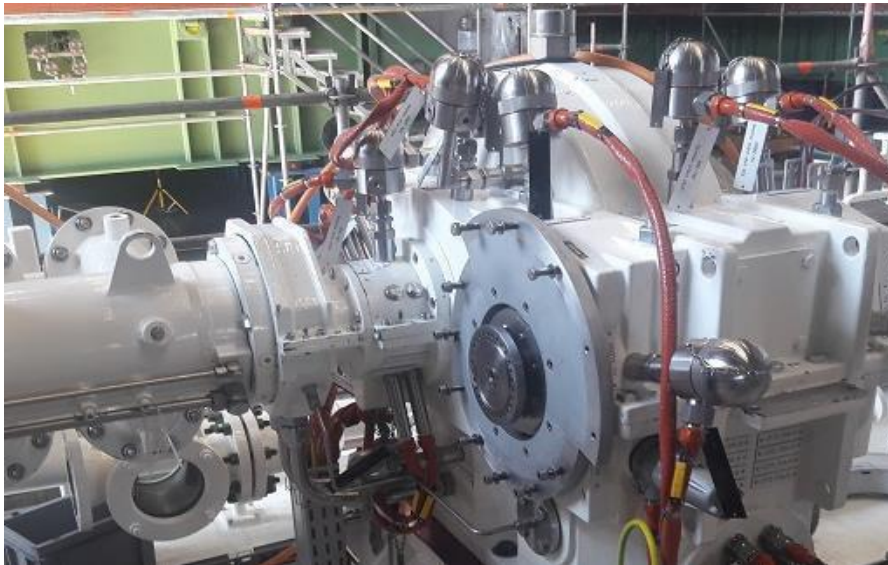
Figure 16 Integral flange coupling fitted in gear box
