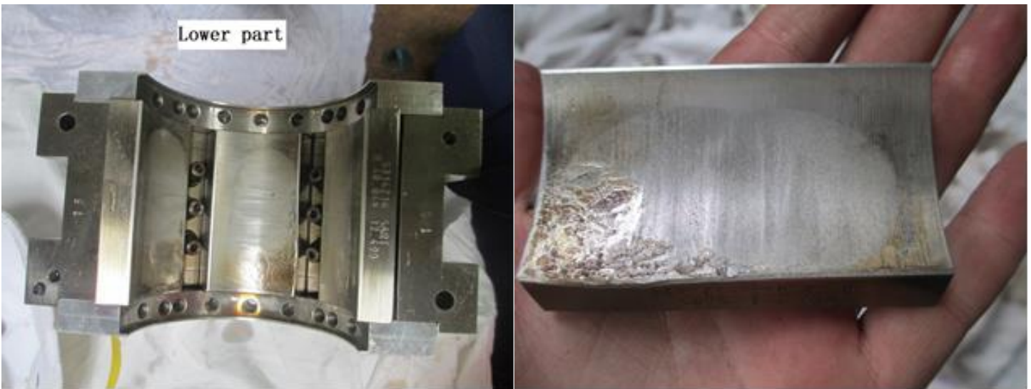
Figure 20: Fourth Stage Bearing Damage for Case Study B
