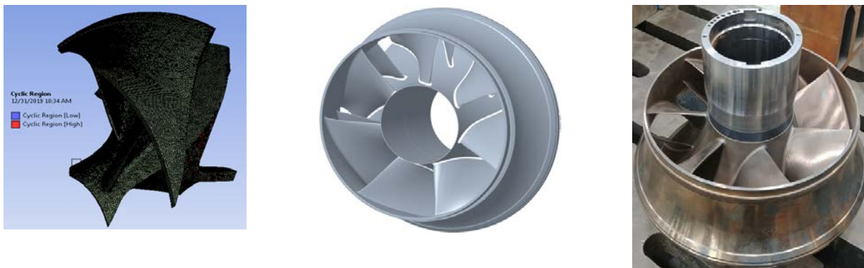
Figure 11. FEA, Solid Model and Test Impeller
