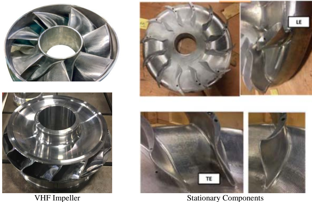
Figure 13. VHF Impeller and Stationary Components
