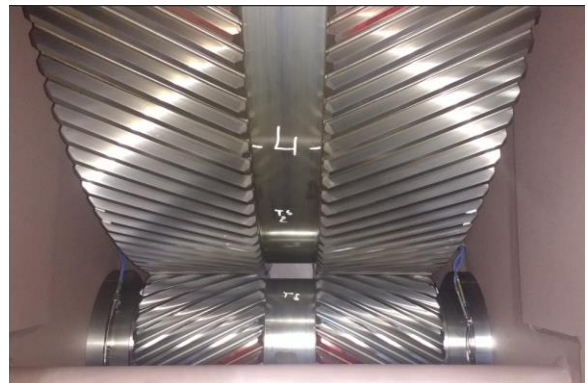
Figure 22: Teeth visual inspection after VG15 test
