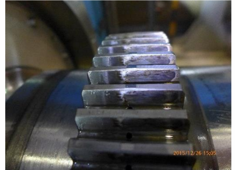
Strange markings on the steam turbine end coupling gear teeth
