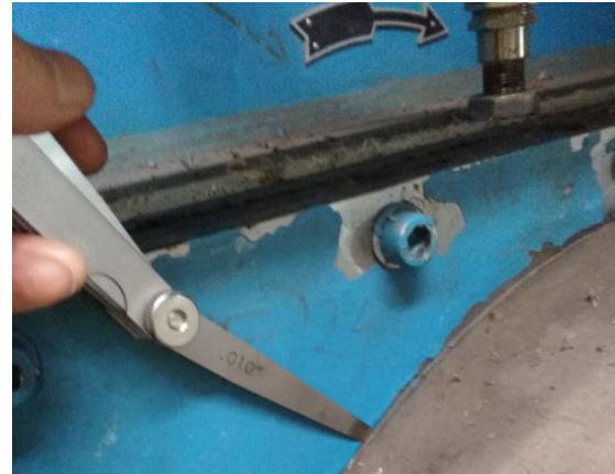
Guard appeared to be pushing against compressor
