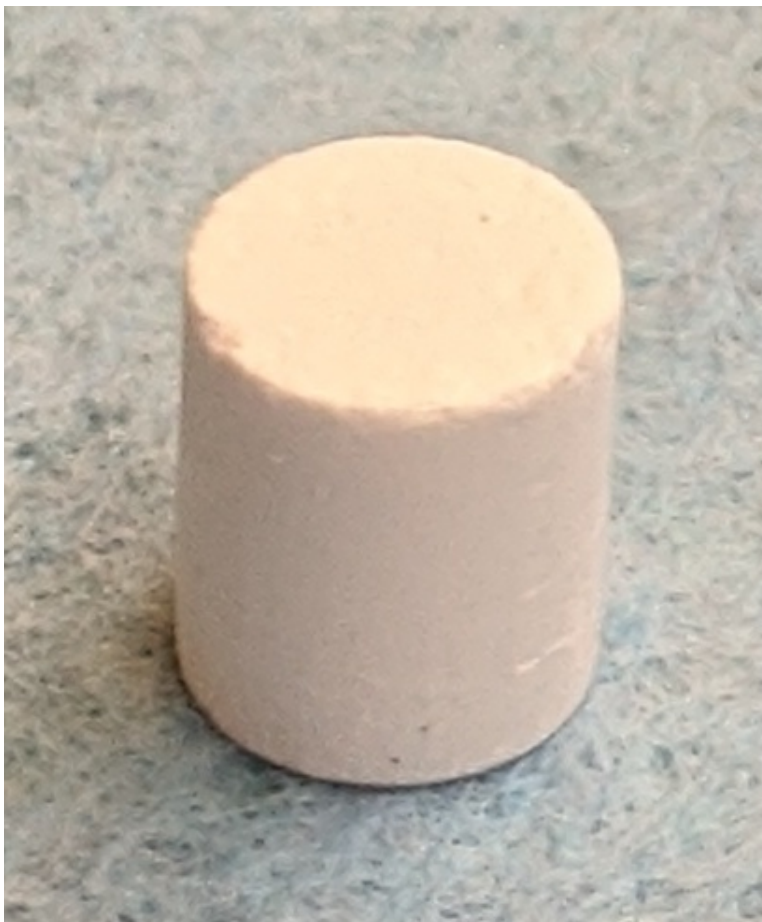
Figure 3.3: Heat treated sample of calcium hydrogen phosphate and calcium carbonate creating tricalcium phosphate.
