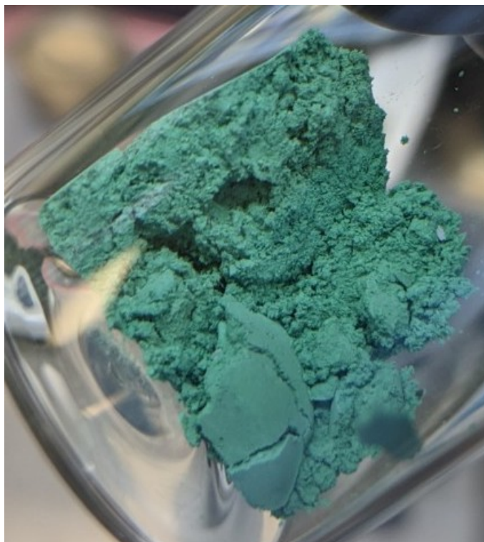
Figure 3.5: Uranium tetrafluoride converted from uranium oxide using ammonium bifluoride.
