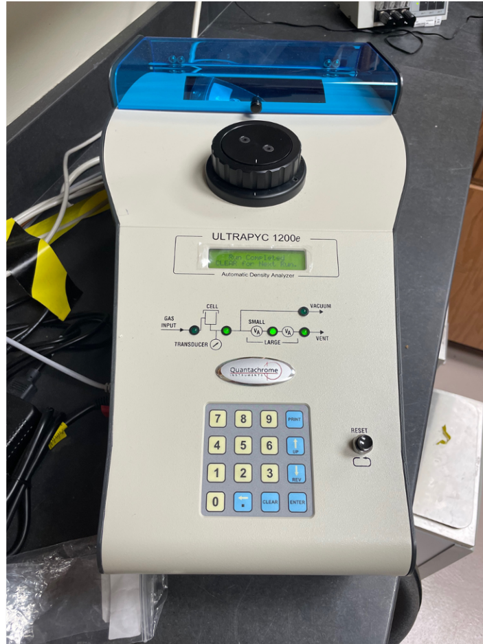
Figure 3.19: The Ultrapyc 1200e used to obtain densities of the FAp waste forms.
