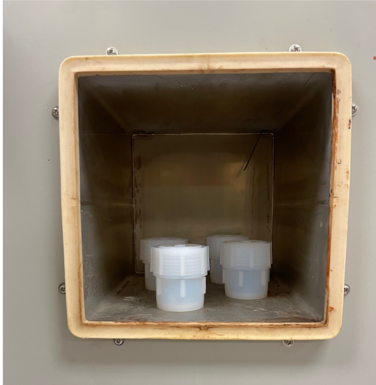
Figure 3.14: Savillex vessels inside the Yamato oven on the final stage of a cleaning process.
