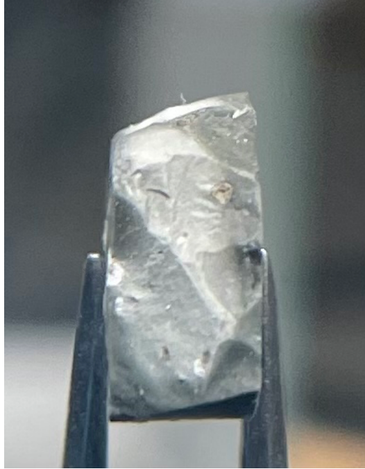
Figure 3.9: Cross section of a pellet created under helium cover gas showing a possible oxidation gradient.
