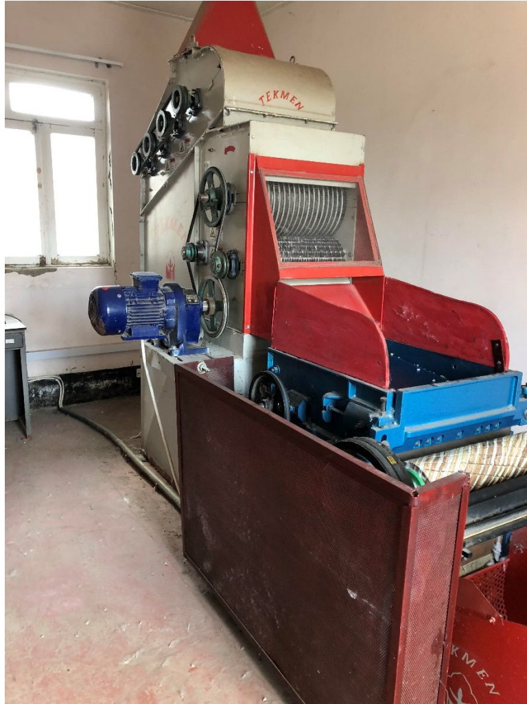
Figure 3.1 Seed cotton samples were ginned on this small-scale roller gin at Imishli, Azerbaijan.
