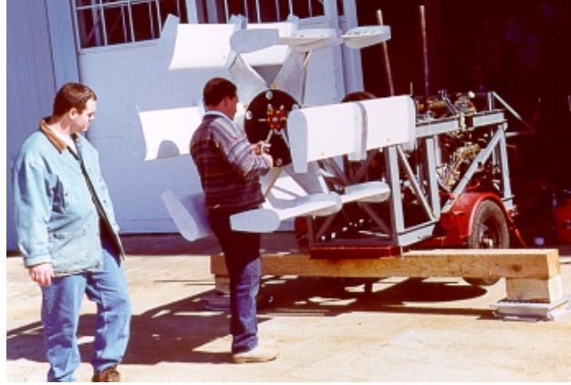
Figure 1.20: Engineers from Bosch working on their cyclorotor test rig[11].
