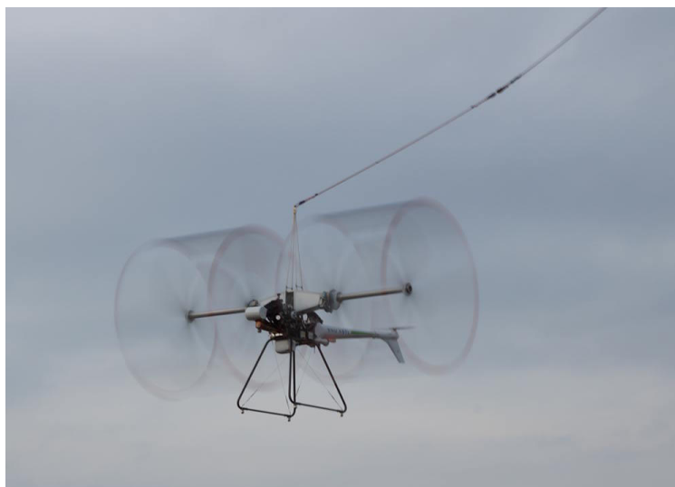
Figure 1.30: 110 kg twin-cyclocopter performing a stable hover with the tether slack[19].
