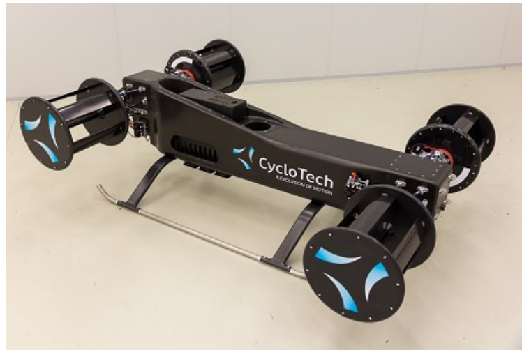
Figure 6.3: 83 kg quad-cyclocopter developed by CycloTech with 4 co-rotating cyclorotors[36].
