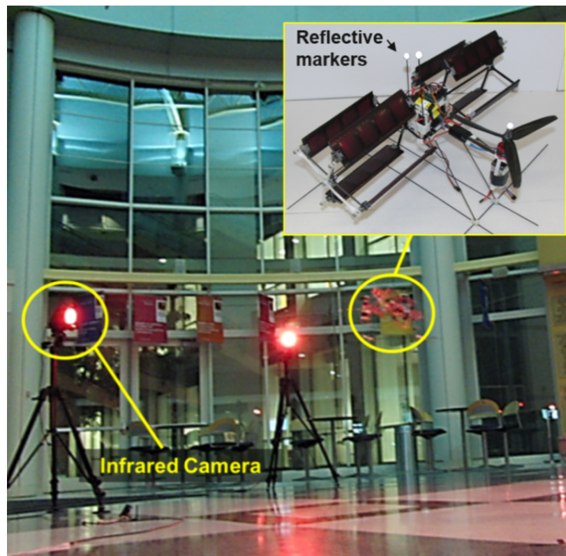
Figure 1.52: Motion capture testing setup for forward flight model determination[27].
