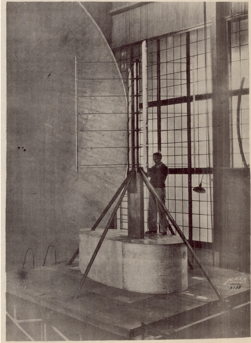
Figure 1.19: Wheatley's 8 ft cyclogiro set up for testing in the 20 ft wind tunnel[10].
