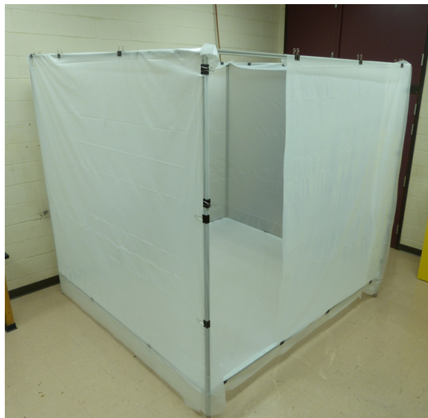
Figure 4.10: Flight space enclosed by Mylar walls to facilitate safe testing.
