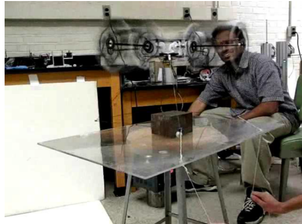
Figure 1.39: Tethered hovering of the quad-cyclocopter[4].
