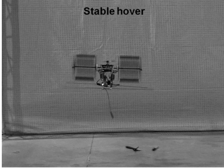
Figure 1.42: First stable, hovering, untethered flight of a cyclocopter based vehicle[22].
