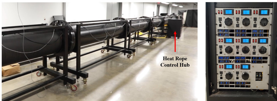
Figure 3.1: The left image is of the SAF assembled within Texas AM’s ALLEMO long-lab. The heat rope control hub can be seen in the left image as well as by itself in the right image.
