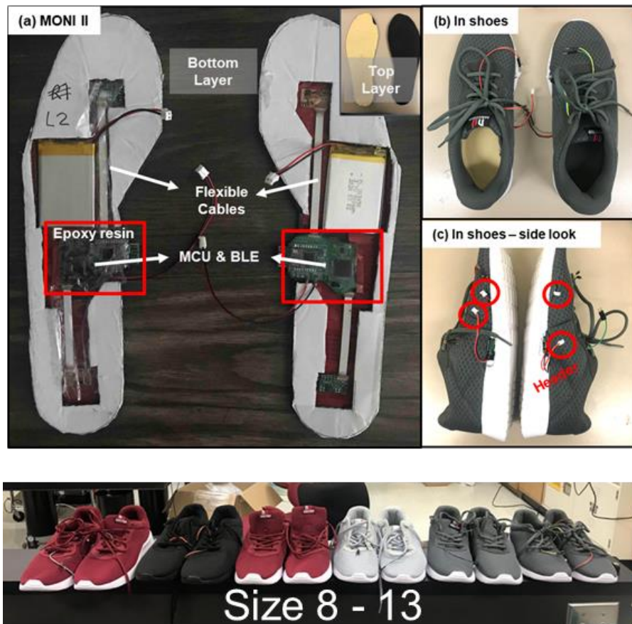
Figure 1.8 The prototype of upgraded MONI (size 8): (a) the bottom layer (the foam with electronics), and the top layer (the high-density textile foam); (b) the top view and (c) the side view inside a pair of MONI inserted in shoes.
