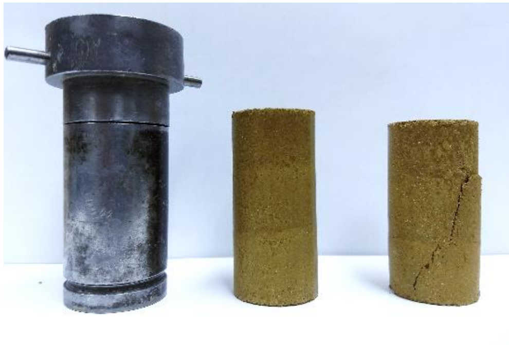
Figure 5.2 Specimen mold, a typical miniature specimen after compaction and after UCS testing.
