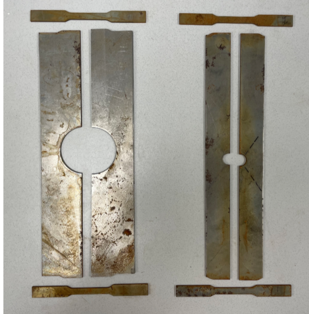
Figure 3.7: Blanked edge specimens post EDM cutting.
