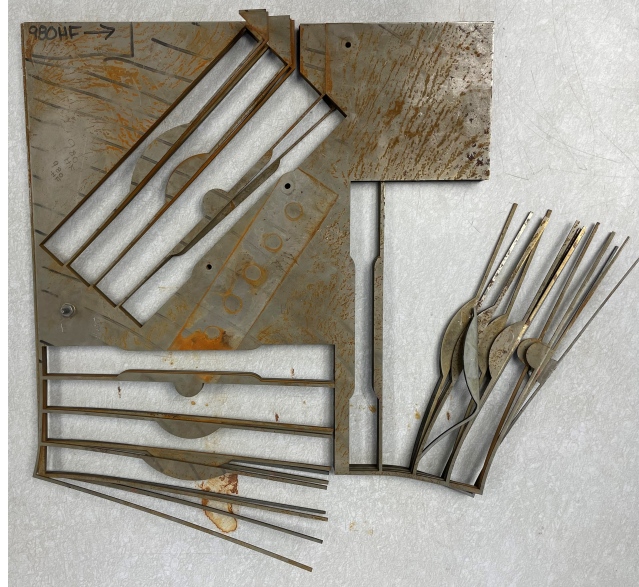
Figure 3.4: Stock plate for machined edge specimens post EDM cutting.
