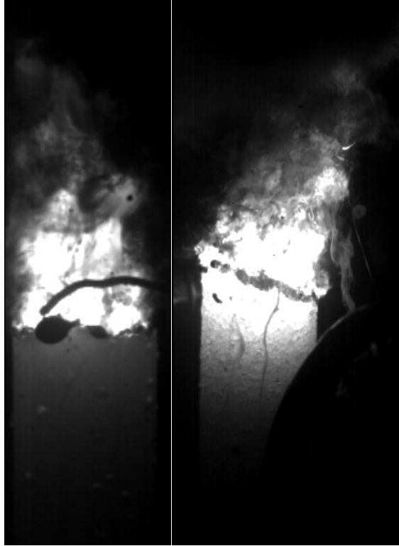
Figure 4. Left: Image of AP/HTPB propellant burning linearly in the axial direction. Right: Image of AP/HTPB propellant burning at an angle in the axial direction.
