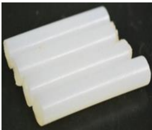
Figure 12. Hand-extruded propellant samples cut to approximately 1-inch in length.
